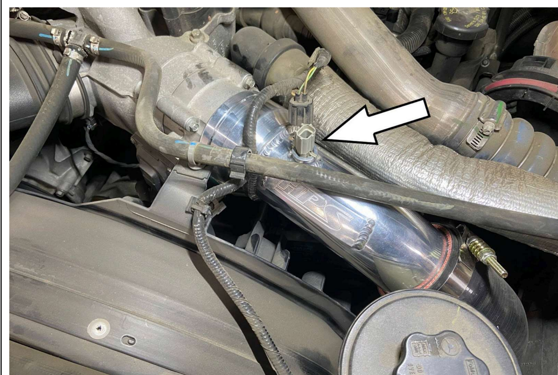
16. Secure the temperature sensor onto the HPS charge pipe and then reconnect the harness.
