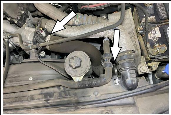
3. Loosen the two hose clamps securing the factory charge hose located at the throttle body and the intercooler.
