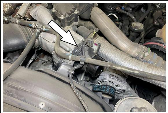
5. Lift the retaining clip to disconnect the quick-connect fitting at the throttle body and remove it from the vehicle.
