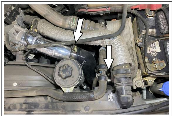
11. Position the charge pipe and the charge hose so that there is proper clearance around and along the product. Then tighten both spring loaded T-bolt clamps.
