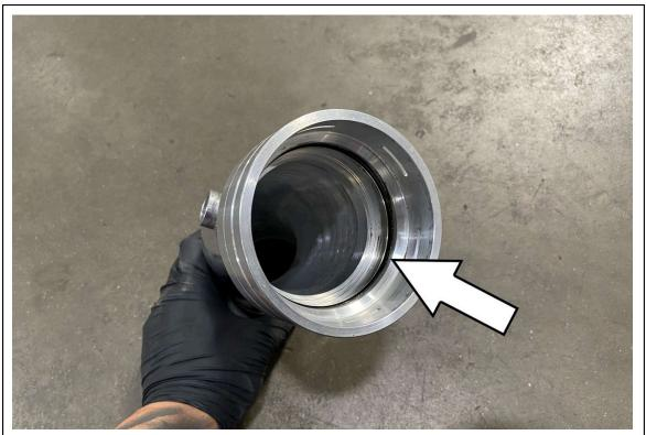
9. Place the provided O-ring into the groove on the HPS charge pipe.
