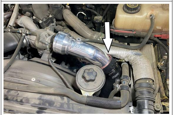
10. Insert the HPS charge pipe into the couple first, then onto the throttle body.
