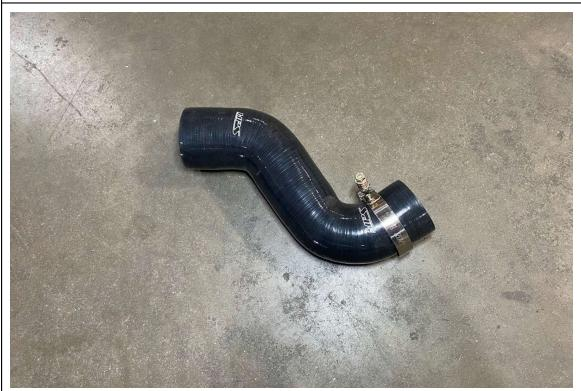
6. Slip the provided 73mm-81mm spring loaded T-bolt clamp onto the smaller side of the HPS charge hose.
