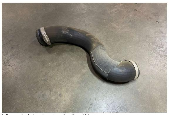
4. Remove the factory charge hose from the vehicle.
