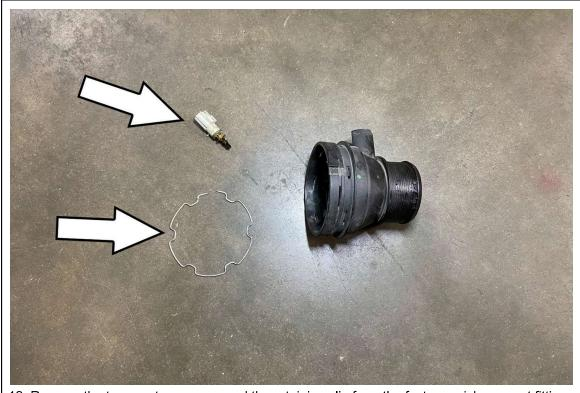
12. Remove the temperature sensor and the retaining clip from the factory quick-connect fitting.
