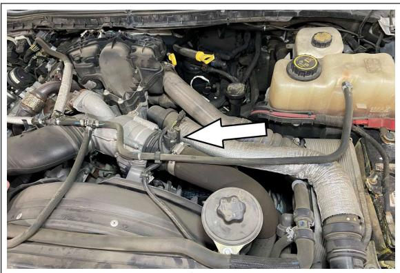
2. Disconnect the temperature sensor on the factory charge pipe.
