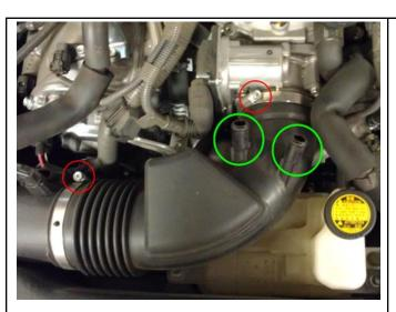
1. Remove engine cover and disconnect the two breather hose on the factory intake tube. Then loose the two hose clamps one both ends of the tube using a 10mm wrench or a Phillips screwdriver.
