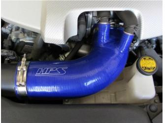
2. Slide the clamps on to the silicone intake tube. Make sure the bigger clamp is on the throttle body side. Install the hose on to the air box side first then to the throttle body. Next tighten the two clamps, reinstall the breather hose and snap the engine cover back on.
