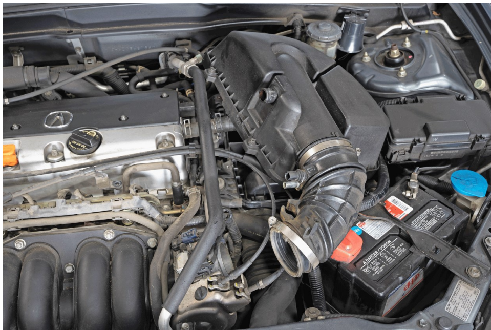
6. Remove the intake assembly along with the upper air box from the vehicle.
