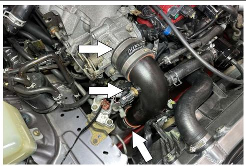
6. Slip the HPS intercooler pipe with couplers over the throttle body and lower intercooler pipe before tightening all four clamps. Install the intake air temperature sensor onto the HPS pipe using the original O-ring and then plug in the sensor harness.
