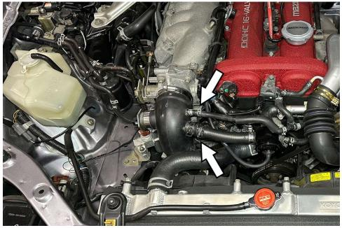
3. Disconnect the vacuum hose and the blow off valve. Remove the factory throttle body intercooler pipe.
