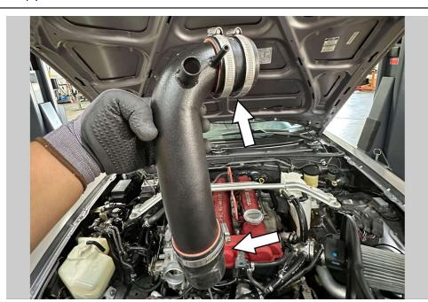
4. Secure the provided clamps and couplers onto the HPS intercooler pipe. The straight coupler will be installed to the throttle body end and the reducer coupler will be installed on the end that will connect to the lower intercooler piping.
