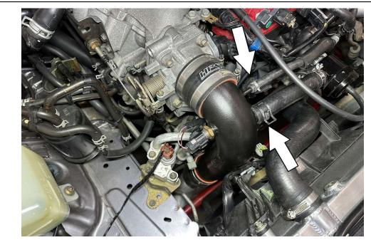
7. Connect the vacuum hose and the blow off valve to the HPS intercooler pipe.
