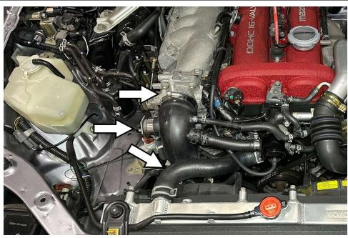
2. Uninstall factory the throttle body intercooler pipe by loosening the upper and lower clamps. Then, unplug and uninstall the intake air temperature sensor.
