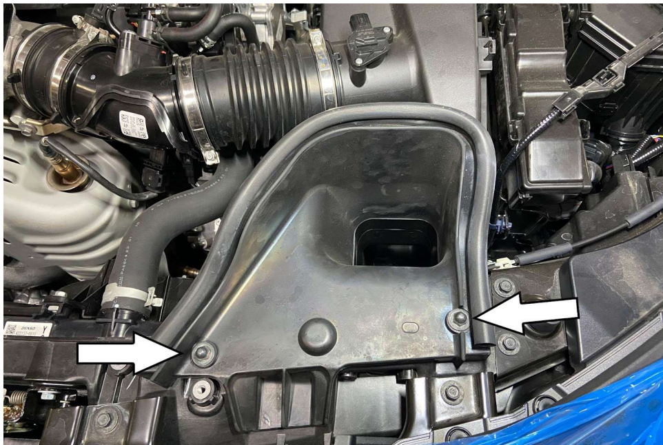
6. Remove the two 10mm bolts securing the factory air duct.
