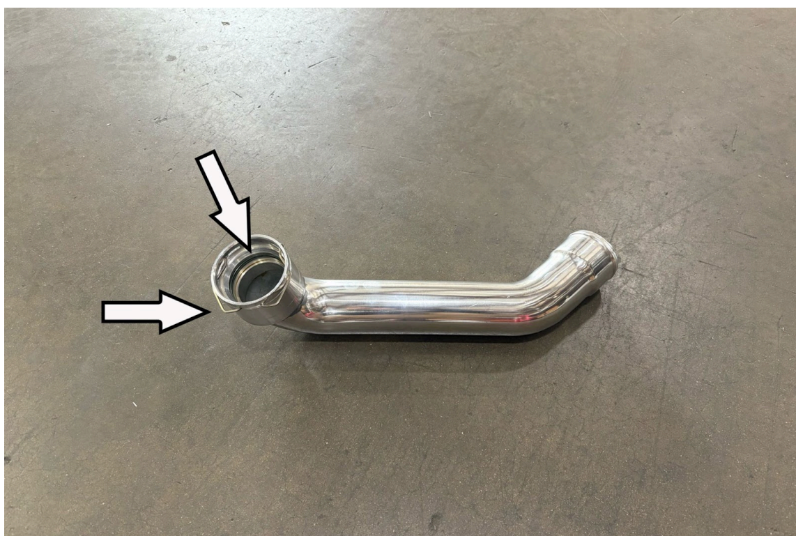
26. Insert the green factory O-ring and retaining clip into the quick-connect on lower HPS charge pipe.
