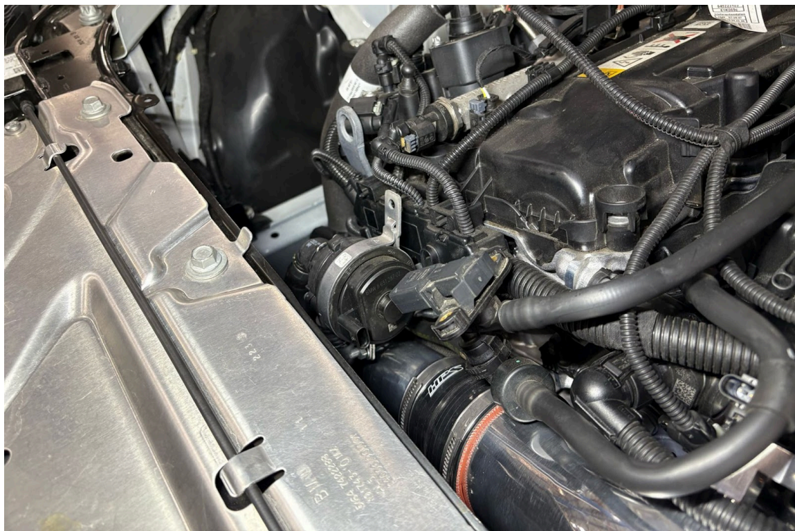
36. Secure the coolant pump assembly back onto the bracket.
