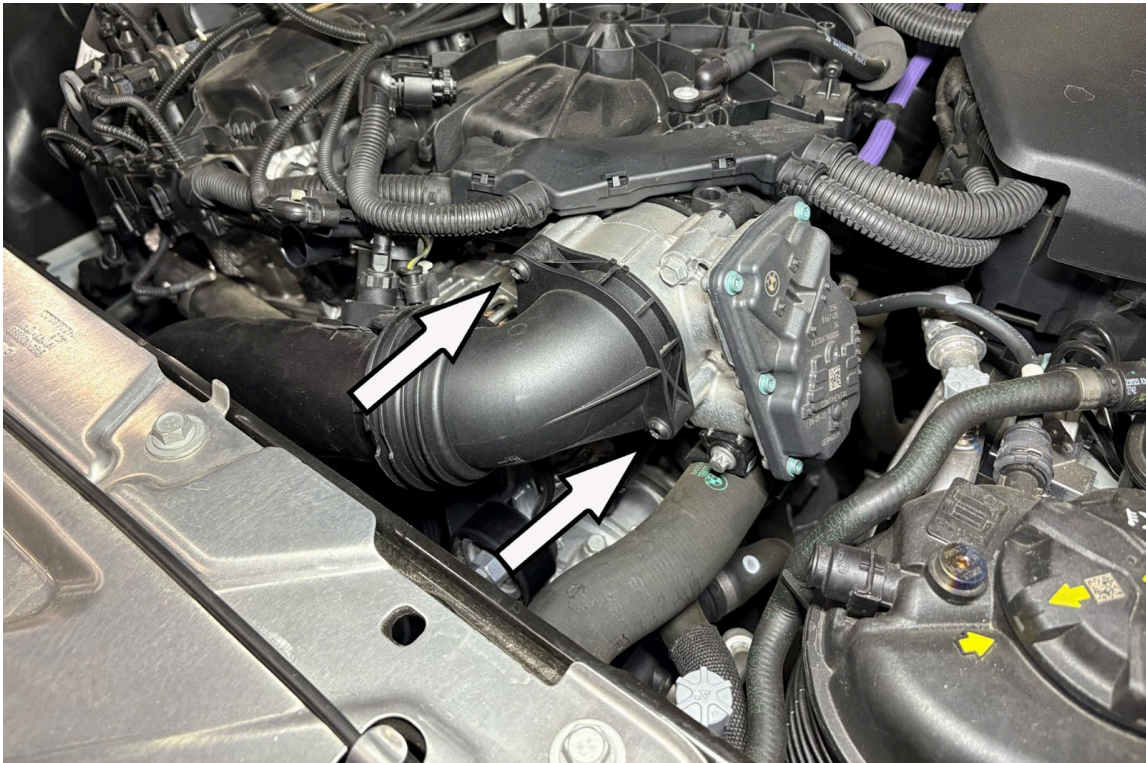
20. Remove the two bolts securing the charge pipe to the throttle body.
