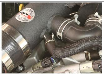
14. Reinstall the stock breather hose into the intake.
