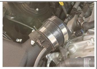
10. Install the coupler and t-bolt clamps onto the air box.
