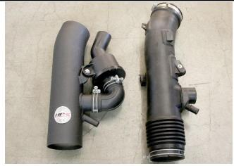
11. **[ For Kit # 27-559 ONLY ]** Remove and switch the stock sound generator onto to the HPS intake pipe. Reuse the factory bolt to secure the sound generator.
