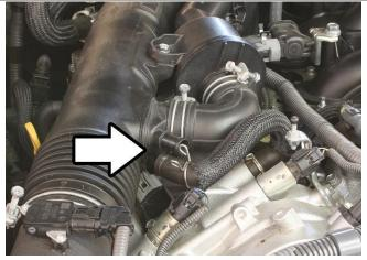
4. Push back the clamp holding the breather hose then remove the breather hose from the factory intake tube.
