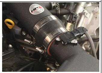
13. Connect the opposite end of the intake pipe to the air box.
