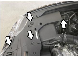
3. Release the four rivets by pushing the center of the rivets then remove the plastic panel covering the air box.
