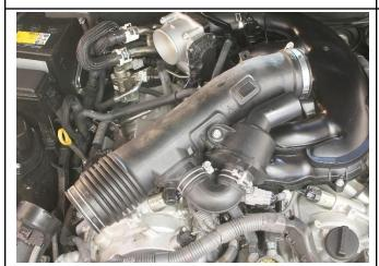
8. Disconnect the intake tube from the air box and the throttle body and remove the intake tube.
