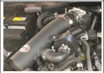
12. Insert the intake into the coupler on the throttle body. (Picture showing kit # 27-559 intake pipe)
