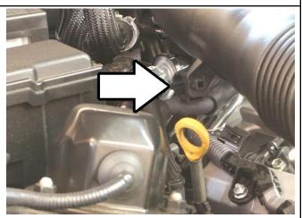
7. Unclip the hose from the bracket on the bottom intake tube.
