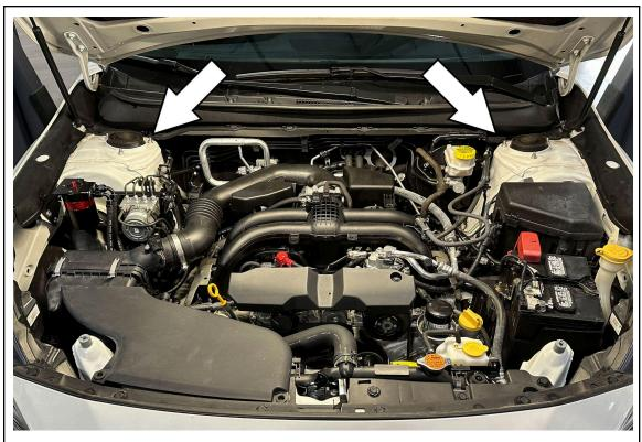
2. Remove the (6) original nuts on the strut tower.
