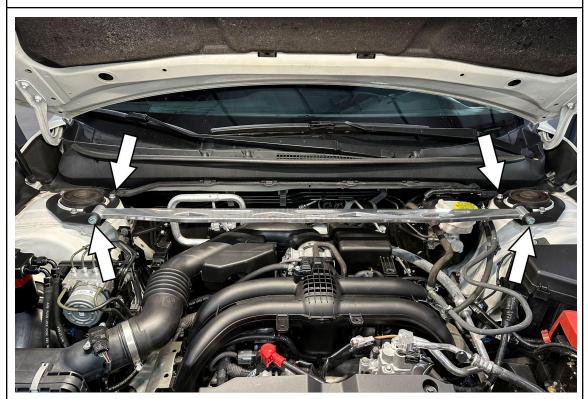
6. Fasten the (6) original strut tower nuts to 14.5 ft-lbs. Then, fasten the (2) Allen head bolts on each side of the strut bar to 86 ft-lbs.
