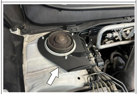
4. Install the provided strut bar brackets on top of the washers that were installed in step 3.
