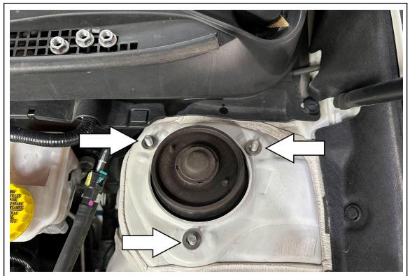
3. Install the provided (6) oversized washers onto the strut mount studs. There are (3) on each side.
