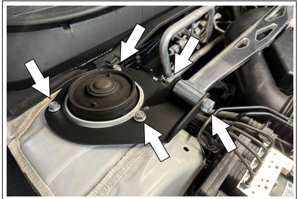
5. Loosely reinstall the original strut tower nuts on both strut towers. Loosely install the HPS strut bar using the provided (2) Allen head bolts and (2) flange nuts.
