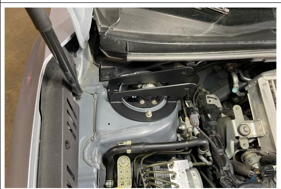
4. Loosely install bracket 431-116-R onto the passenger side strut tower using the factory nuts removed in step two.
