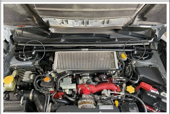
6. Loosely install the center strut bar using the two provided M12 bolts and two M12 flanged nuts. Once the bar and brackets are properly positioned, secure all of the nuts and bolts.
