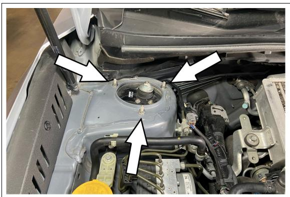
2. Remove the three nuts from the passenger side strut tower and set aside.
