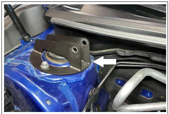
3. Place the strut bar brackets onto both of the strut towers.
