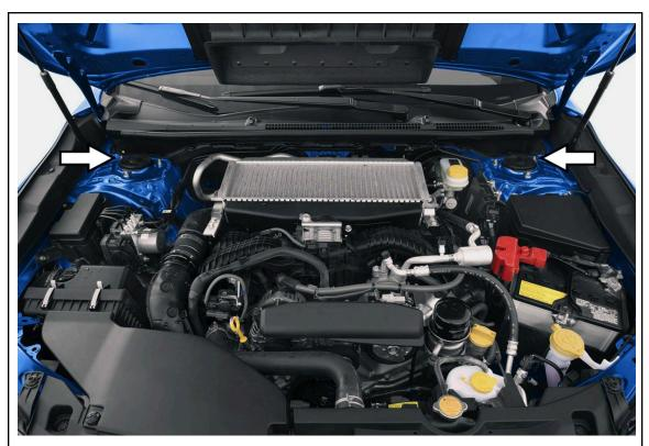
2. Loosen and remove the six strut mount nuts on strut towers. Set the nuts aside to be reused in a later step.
