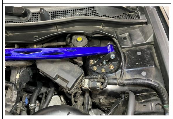
6. Once the bar and brackets are properly positioned, secure all of the nuts and bolts.
