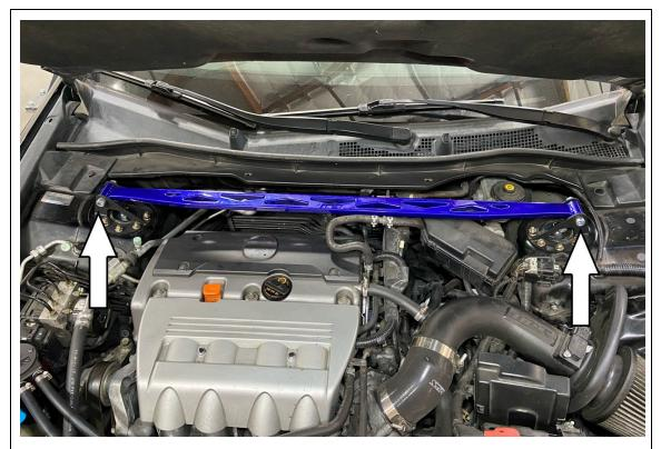
5. Loosely install the center strut bar using two of each provided M12 bolts and M12 flange nuts.
