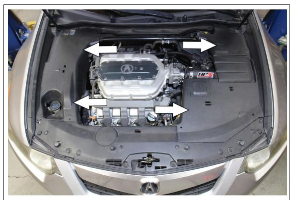
2. On V6 models, the plastic side panels will need to be removed from the vehicle.
