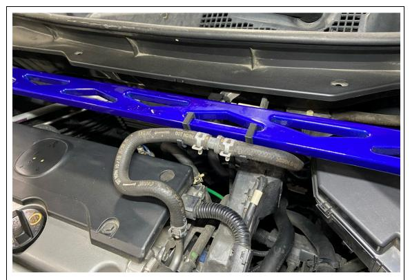
9. Secure the vacuum hose onto the brackets.
