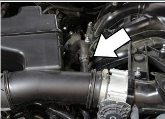
3. Using a pair of pliers, pinch and move the hose clamp from the breather hose, then remove the breather hose from the intake tube.
