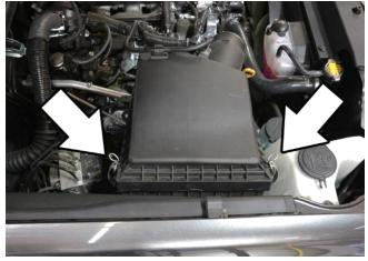
6. Unbuckle the 2 clips securing the upper part of the air box assembly.
