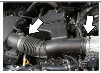
4. Loosen the hose clamp securing the throttle body and the air box, then locate the Mass Air Flow sensor harness clip on the resonator.
