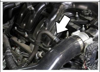
9. Re-install the breather hose onto the HPS intake.
