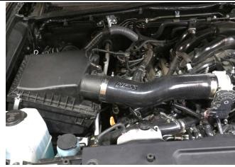
8. Insert the HPS intake onto the air box side first then onto the throttle body side, re-clip the upper part of the air box, and finally adjust the HPS intake to the proper position.
