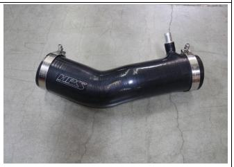
7. Install the T-bolt clamps onto the HPS silicone intake, but do not tighten the t-bolt clamps at this time.
