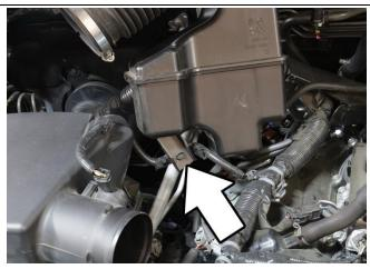
5. Remove the MAF sensor harness clip from the resonator to remove the stock intake tube from the vehicle.
