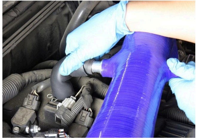
11. Connect the valve cover breather hose onto the back port on the intake tube. The stock spring clamp will be used to secure the hose to the breather port.
