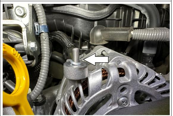
6. Install the provided 25mm long set screw and M6 split lock washer at the mounting hole where the original bolt was removed in step 2. Thread the set screw until it sits flush with the bottom of the mounting hole.
