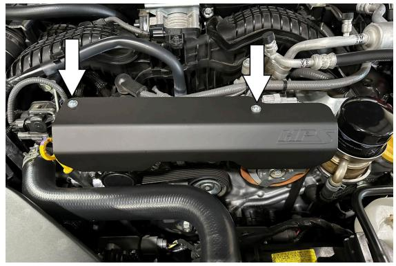
8. Install the HPS belt cover using the two smaller M6 washers and two button head bolts.
