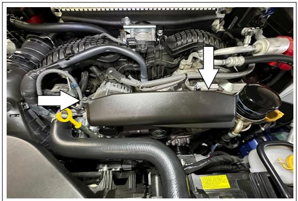
2. Remove the original belt cover mounting bolt. Pull up on the plastic push pin and remove the original belt cover.
