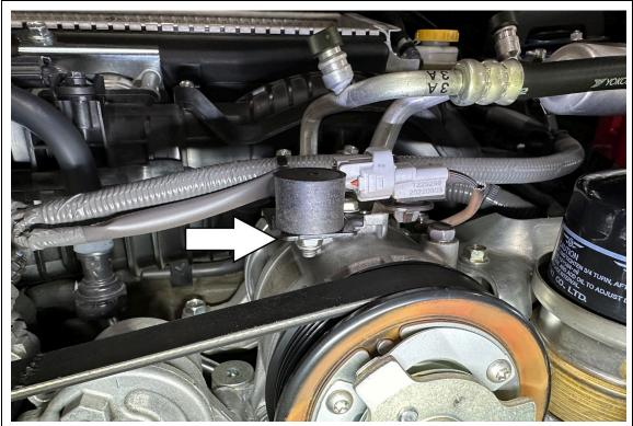
5. Install the pre-assembled vibration mount where the original rubber grommet was mounted.
