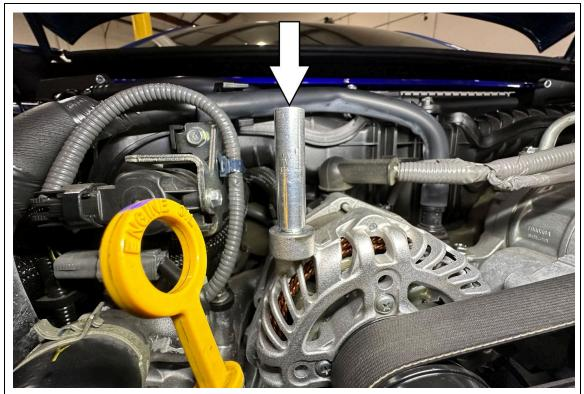
7. Fasten the provided 51mm long spacer onto the previously installed stud and split washer. Make sure to tighten down the spacer until the split lock washer is flat.
