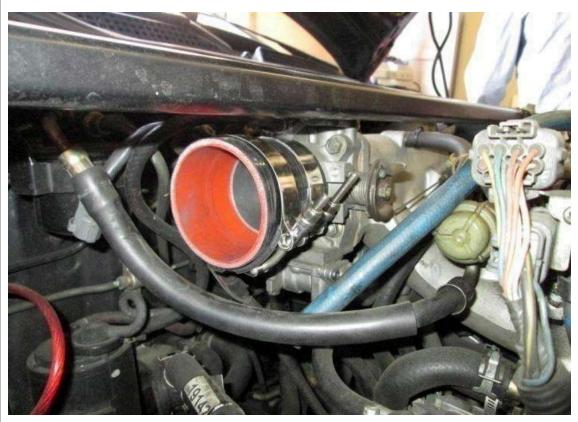
4. Slip the silicone coupler and T-bolt clamps onto the throttle body. Only secure the clamp on the throttle body end at this time.
