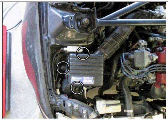
3. Remove the three bolts securing the airbox to remove the airbox and air intake hose from the engine bay.
