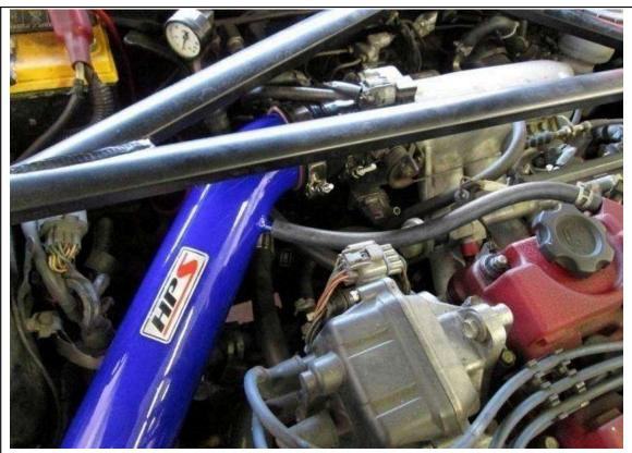
5. Slide the HPS intake pipe onto the coupler at the throttle body but do not tighten the second clamp at this time. Install the breather hose included in the kit by pushing one end onto the bung of the HPS intake. Reuse the factory clamp to secure the other end to the valve cover.
