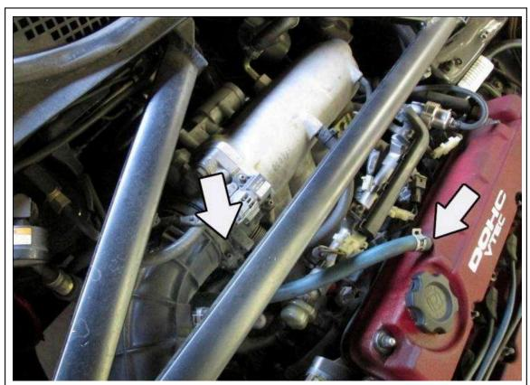
2. Loosen the clamp on the factory air intake hose at the throttle body and disconnect the breather hose from the valve cover.
