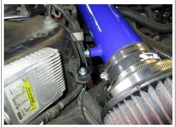
6. Install the rubber mount and intake bracket using the hardware included. Attach the HPS Air Filter to the end of the intake.
