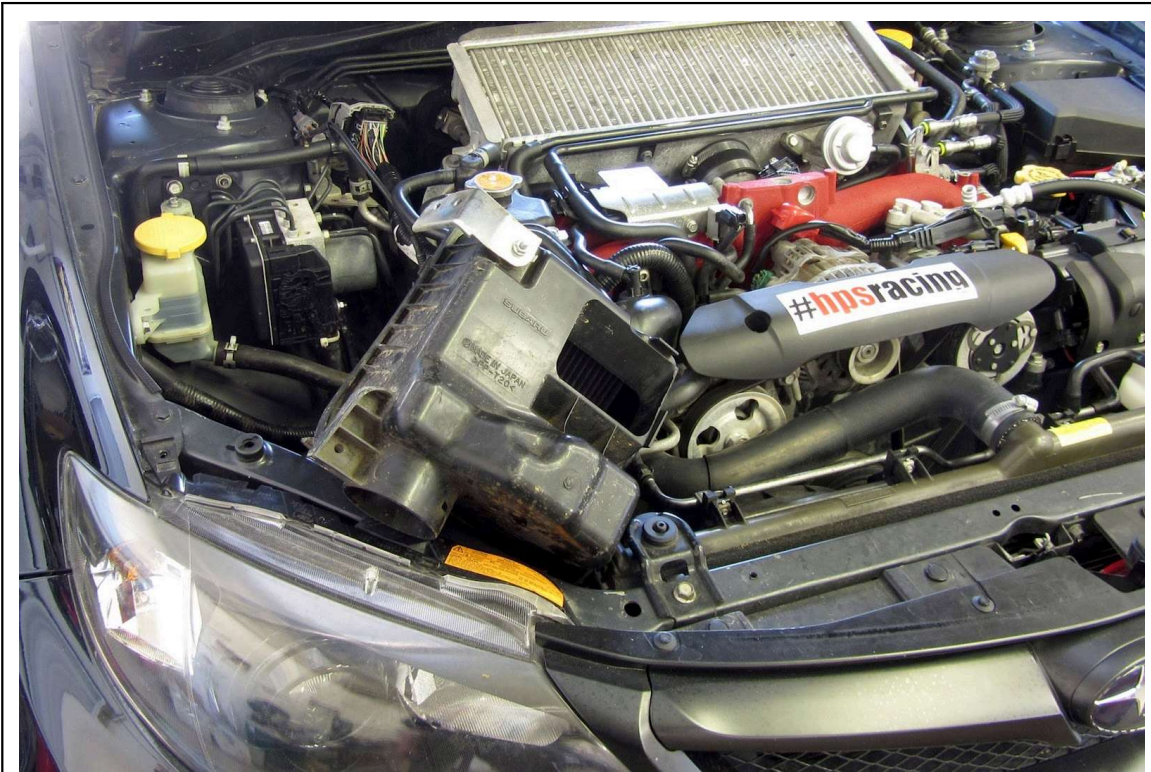
9. Remove the lower air box assembly from the engine bay.
