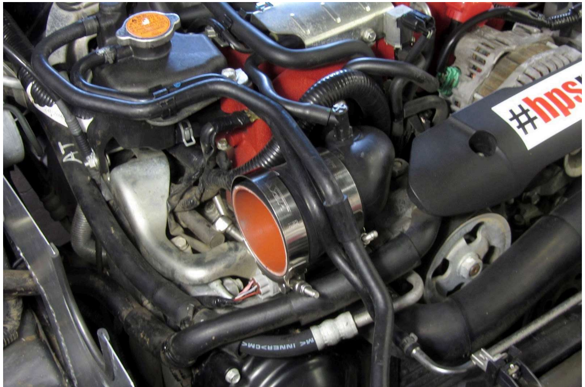
16. Install the reducer coupler and T-bolt clamps onto the turbo inlet.
