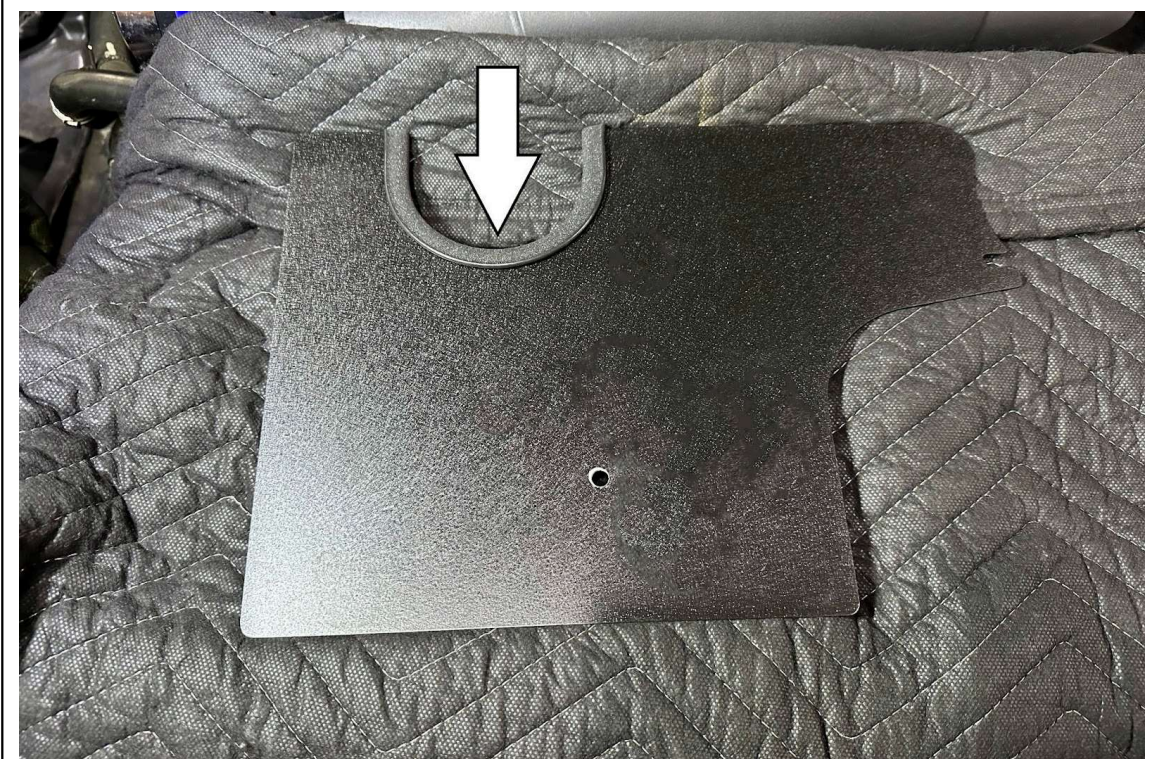
12. Install the thin edge trim onto the heat shield.
