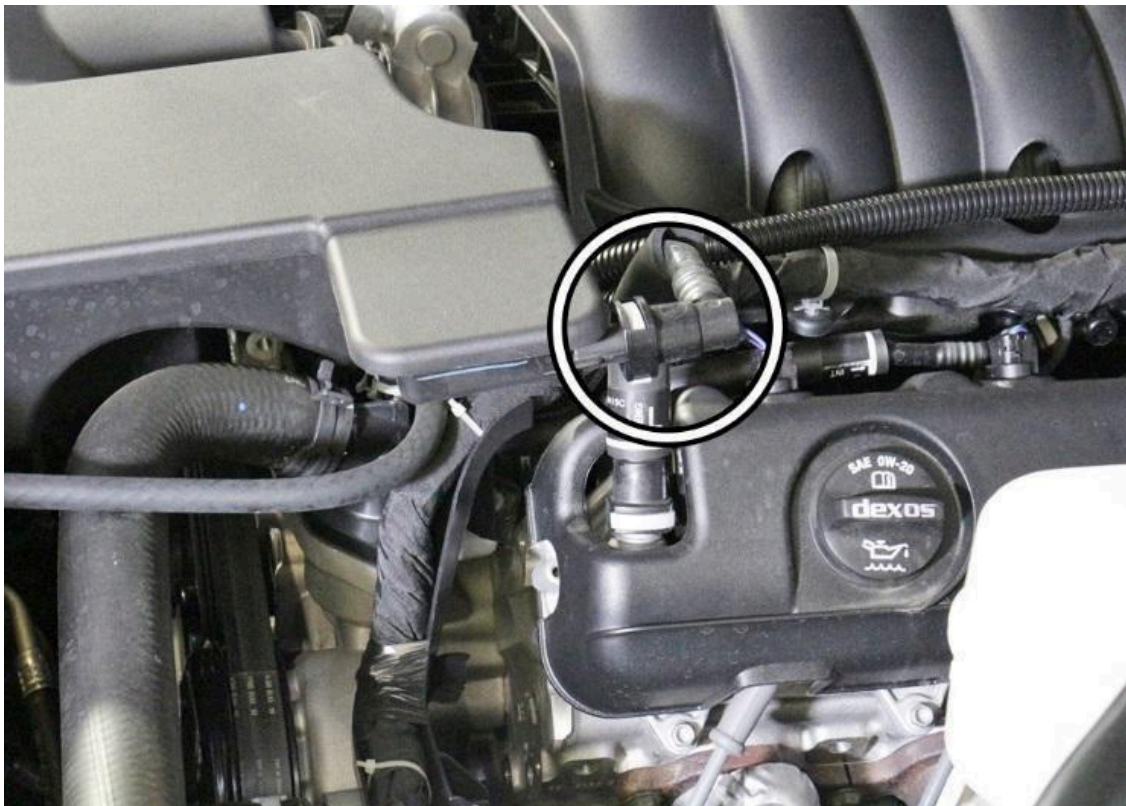
4. Disconnect the breather tube on the other side of the stock intake.
