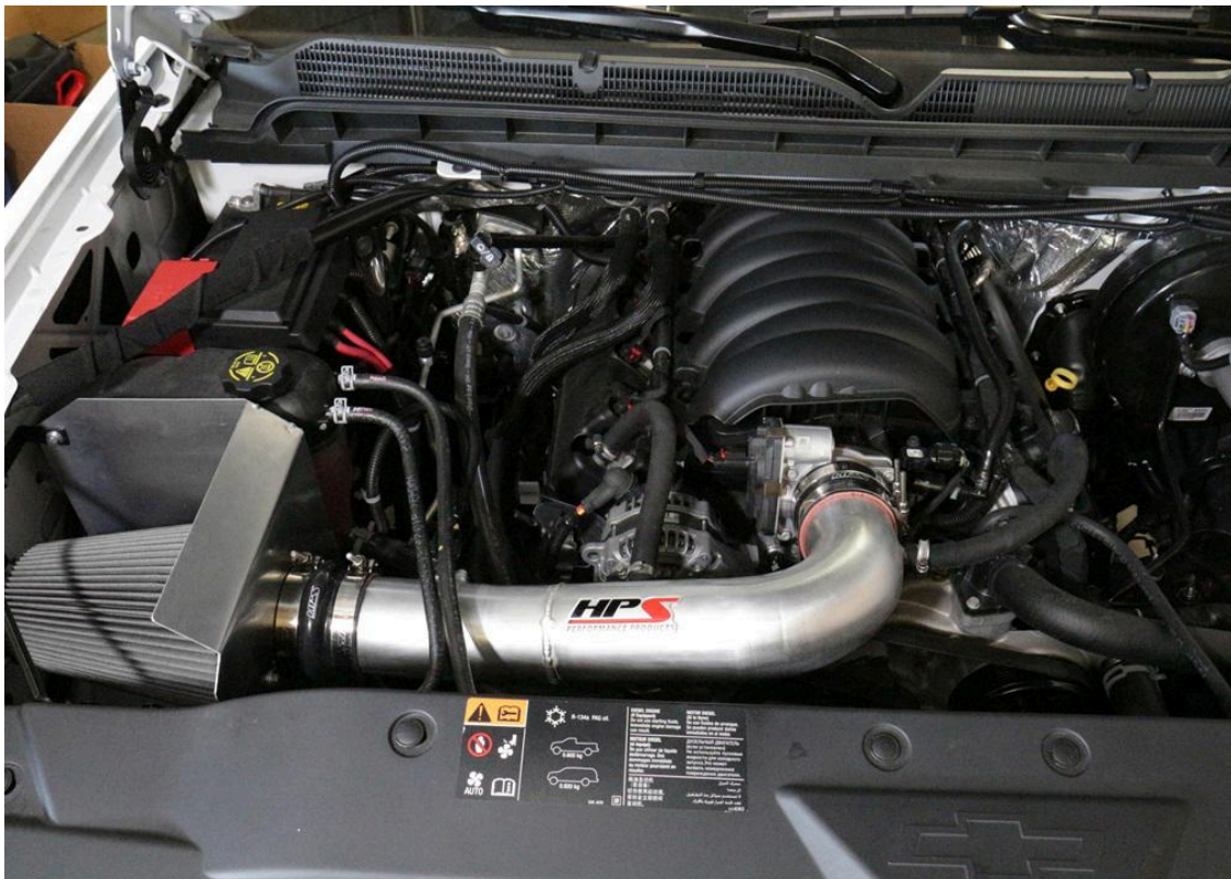
22. Reconnect the MAF sensor connector.
