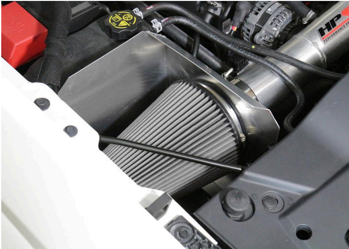
21. Install the provided HPS performance air filter onto the velocity stack.
