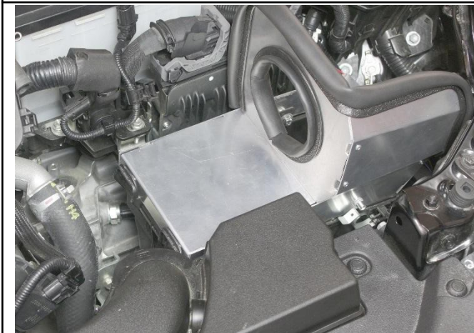
20. Place the heat shield onto the lower air box assembly as shown.
