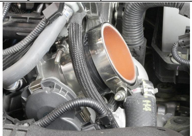
25. Install the silicone reducer coupler onto the throttle body with the small side in first. Only secure the clamp on the throttle body.
