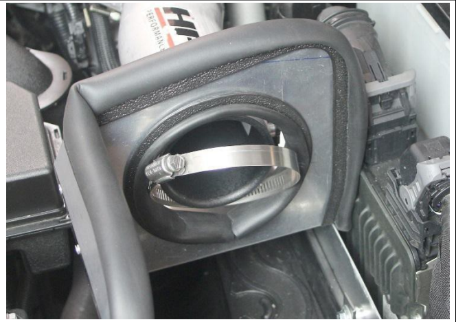
35. Place the clamp through the heat shield opening and onto the intake pipe.
