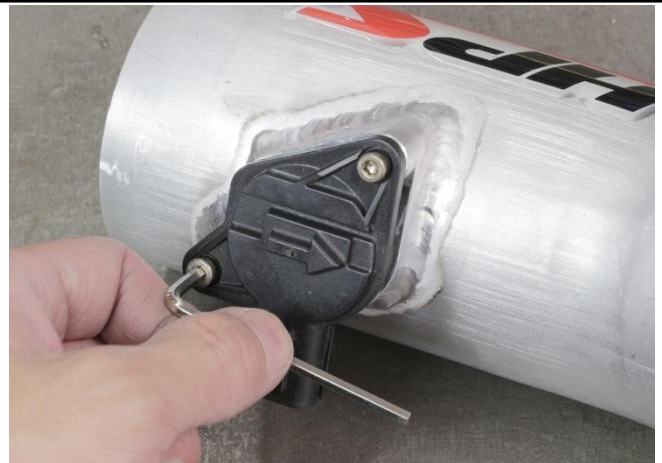
27. Install the MAF sensor onto the HPS intake pipe with the allen screws provided.
