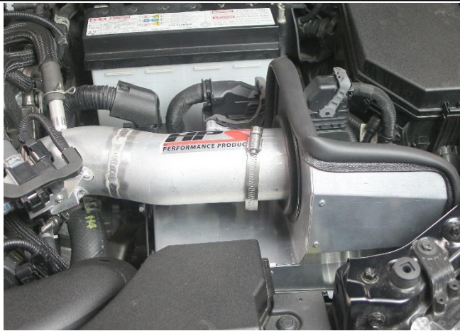
36. Be sure to place the clamp as far in as possible to allow the air filter to seat.
