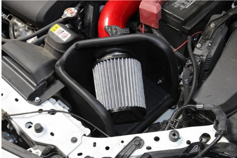
25. Install the provided HPS performance air filter onto the intake pipe.
