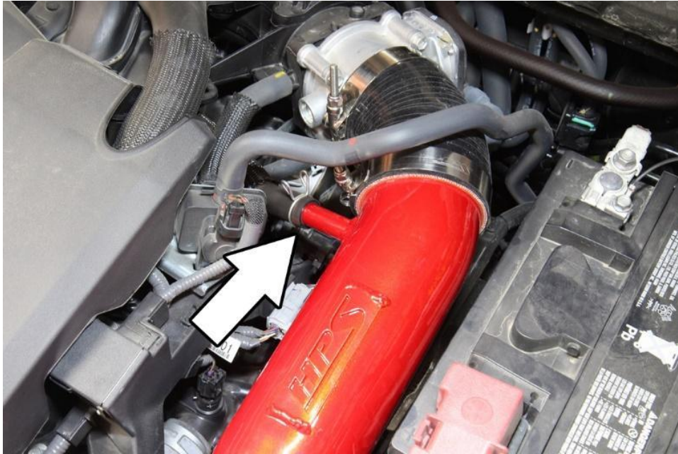
23. Insert and secure the factory breather hose into the intake breather barb.
