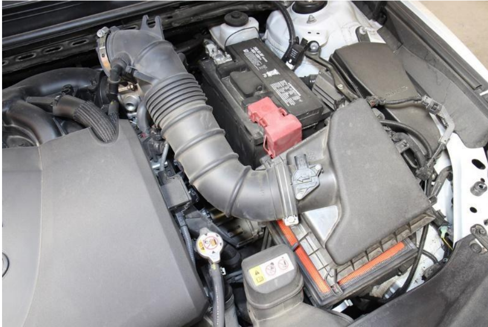
7. Remove the stock intake and the upper air box assembly from the vehicle.
