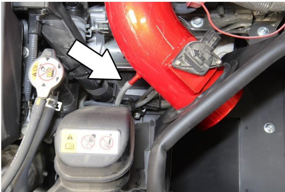
24. Insert and secure the factory vacuum hose onto the intake vacuum barb.
