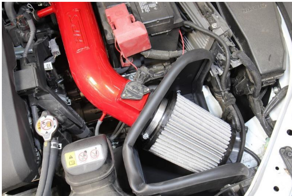
26. Reconnect the MAF sensor harness connector onto the MAF sensor.
