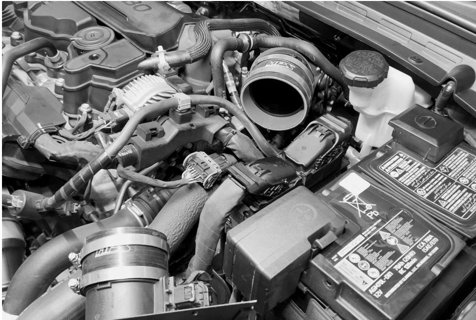
16. Install the couplers onto the turbo inlet and mass airflow sensor housing using the provided EMSC clamps.
