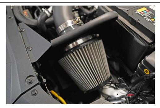
13. Install and secure the provided HPS Performance Air Filter onto the velocity stack.
