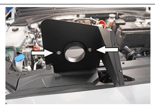
8. Install and secure the velocity stack to the heat shield using the provided M6 bolts (2) and M6 washers (2).
