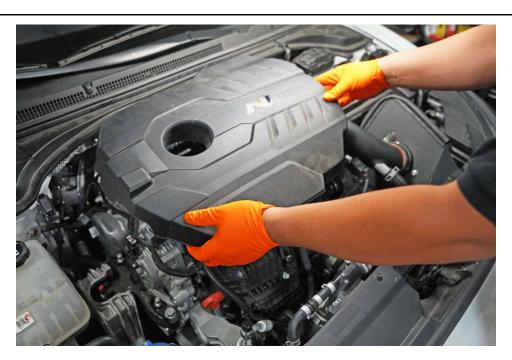
14. Reinstall the engine cover back into the vehicle.
