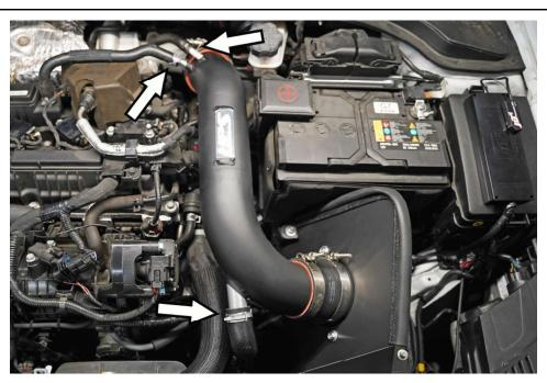
12. Insert and secure the HPS intake pipe into the couplers. Reinstall the vent hoses and the recirculating hose onto the barbs of the HPS intake pipe.
