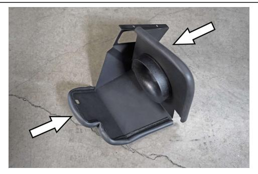
9. Install the provided bubble edge trim onto the heat shield shown at the sections above.
