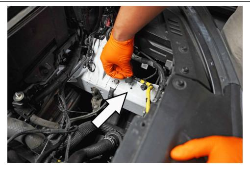
7. Install the other provided  $\frac{1}{2}$ " vibration mount (1) into the factory air box thread.
