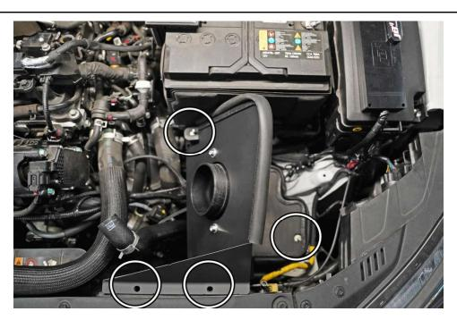
10. Insert and secure the heat shield onto the vibration mounts using the provided M6 nuts (2) and M6 washers (2). Secure the heat shield to the air duct using the factory clips.
