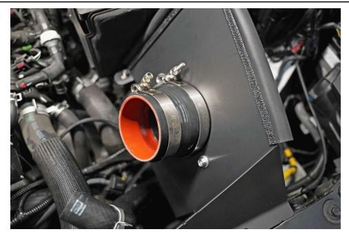
11. Insert and secure the reducer coupler onto the velocity stack along with the provided T-bolt clamps.
