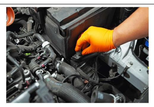
6. Install one provided  $\frac{1}{2}$ " vibration mount (1) into the factory air box thread.
