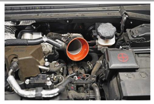
5. Insert and secure the reducer coupler along with the provided T-bolt clamps onto the turbo inlet.
