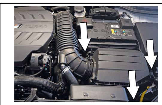
2. Remove the three 10mm bolts securing the air box assembly.
