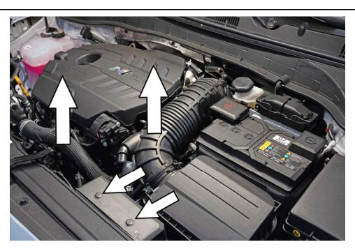
4. Push the center of the retaining clips to release and remove the clips from the factory air duct. Remove the engine cover from the vehicle.
