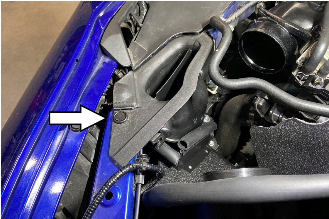
20. Reinstall the factory air duct back into the vehicle.
