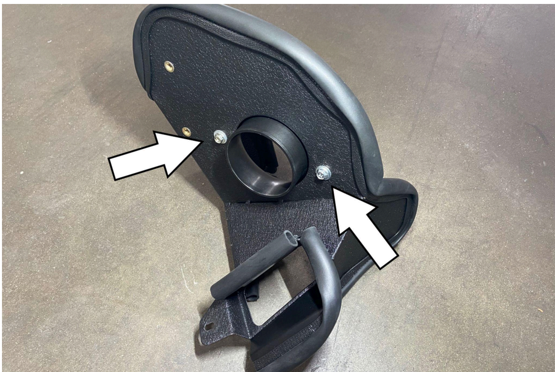
12. Mount the velocity stack onto the heat shield using two provided M6 bolts and washers using a 10mm socket.
