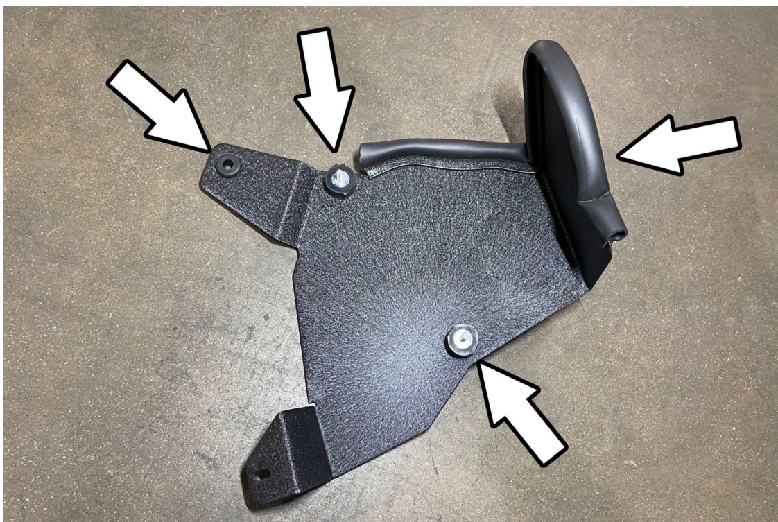
8. Insert the provided grommet into the HPS lower heat shield (shown in top left), then install the 1/2" vibration mounts into the heat shield. Install the bubble edge trim in the area shown above(top right). NOTE* (Bubble edge trim will need to be cut to length)
