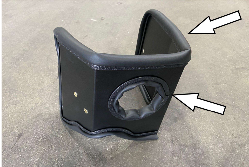
15. Install the provided bubble edge trim onto the HPS heat shield. (Note: bubble edge trim will need to be cut to length. 14.3" for the round opening.)
