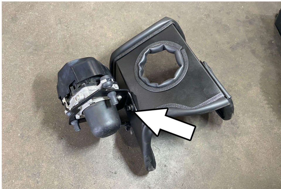
16. Secure the air pump bracket onto the HPS heat shield using the provided M6 x 16mm bolts (2) and washers (2).
