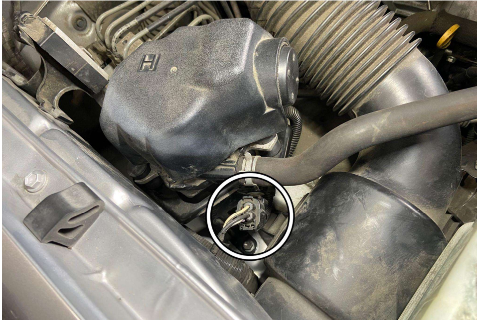
9. Disconnect the air pump electrical harness connector.
