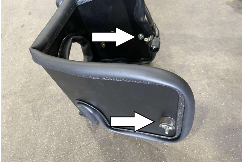
17. Secure the two rubber vibration mounts onto the heat shield from the outside going in using the provided M6 nuts (2) and washers (2).
