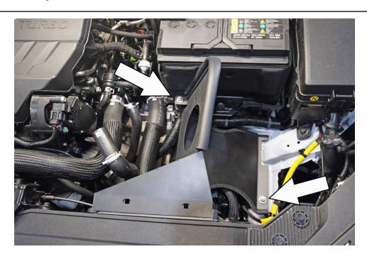
8. Insert and secure the heat shield onto the vibration mounts using the provided M6 nuts (2) and washers (2).
