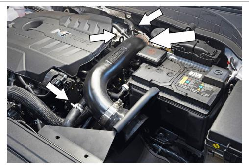
11. Insert the HPS intake pipe into the turbo inlet coupler first, then into the velocity stack coupler. Secure the vent hoses and the recirculating hose onto the HPS intake pipe barbs using the factory retaining clips.
