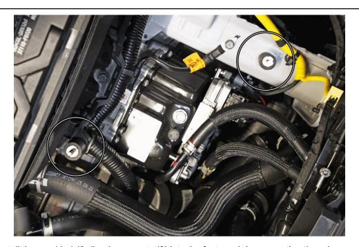
6. Install the provided 1" vibration mounts (2) into the factory air box mounting threads.
