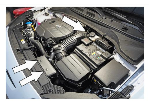
4. Push the center of the retaining clips to release and remove the clips from the factory air duct. Loosen the hose clamp securing the intake hose from the turbo inlet and remove the intake assembly along with the air box from the vehicle.
