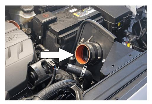
10. Install and secure the reducer coupler along with the provided T-bolt clamps onto the velocity stack.
