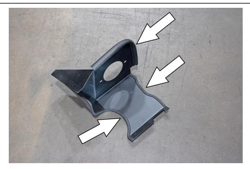
7. Install the provided bubble edge trim along the top of the heat shield. Install the provided thin edge trim along the sides of the heat shield.
