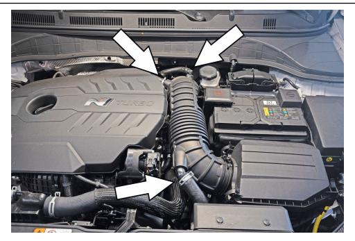
3. Disconnect the vent hoses and the recirculating hose from the factory intake tube.
