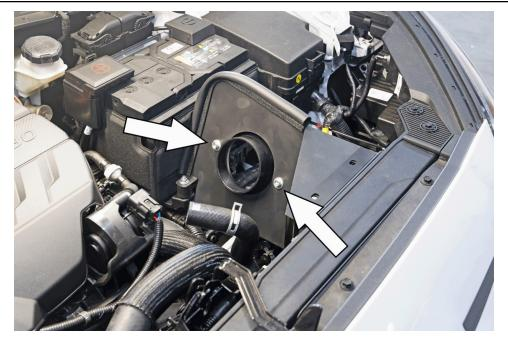
9. Insert and secure the velocity stack onto the heat shield using the provided M6x12mm bolts (2) and washers (2).
