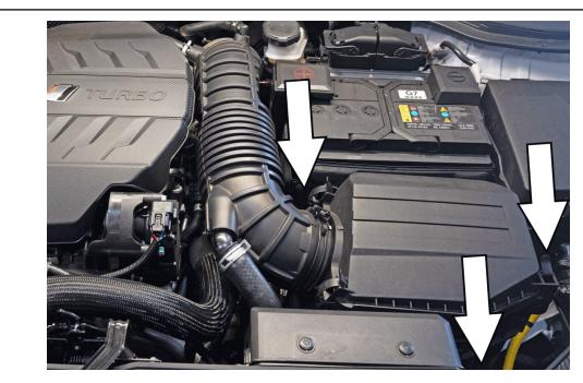
2. Remove the three 10mm bolts securing the air box assembly.
