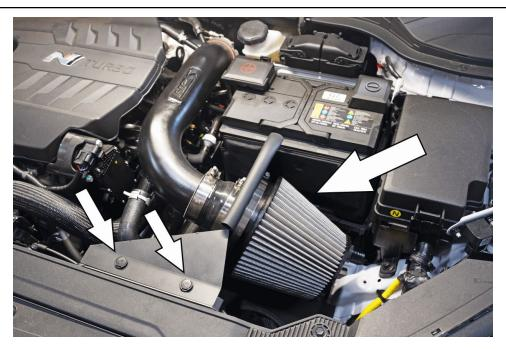
12. Insert and secure the HPS performance air filter. Reinstall the plastic clips to secure the HPS heat shield to the factory air duct.
