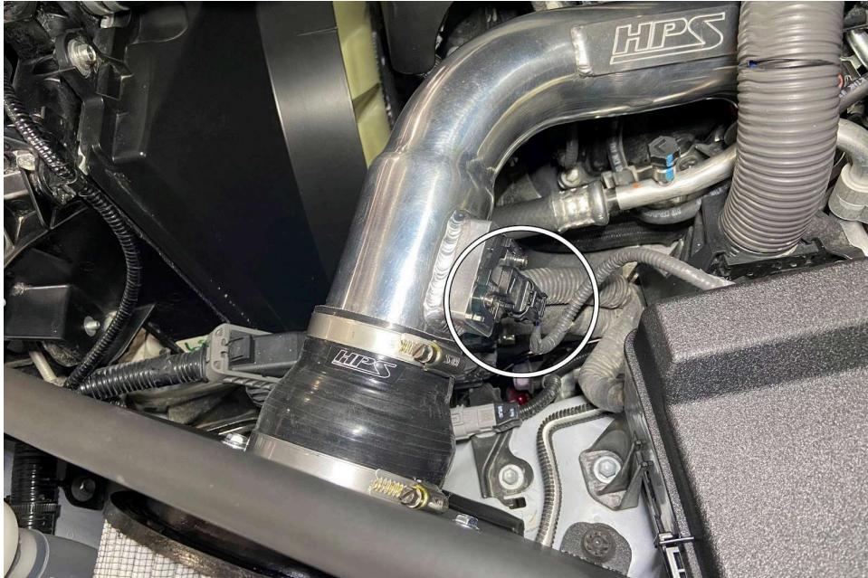
38. Reconnect the mass air flow sensor harness.
