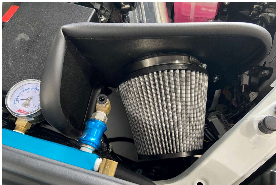
18. Install the HPS Performance Air Filter.
