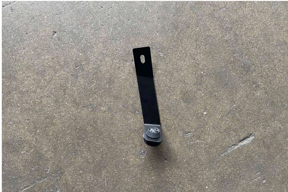
32. Insert factory rubber grommet into the driver side "L" bracket.
