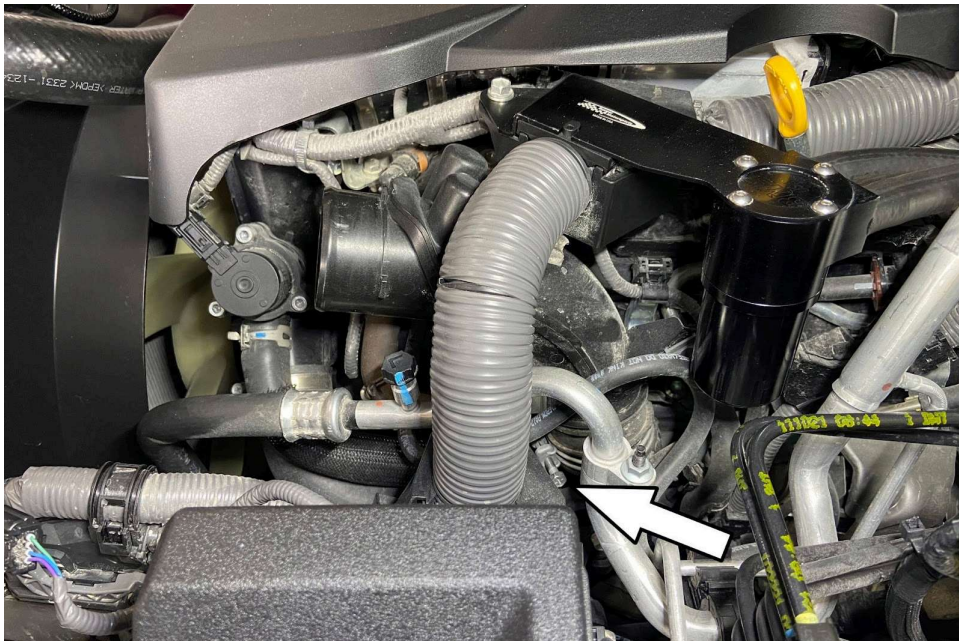
24. Loosen the hose clamp securing the turbo elbow to the turbo and remove it from the engine bay.
