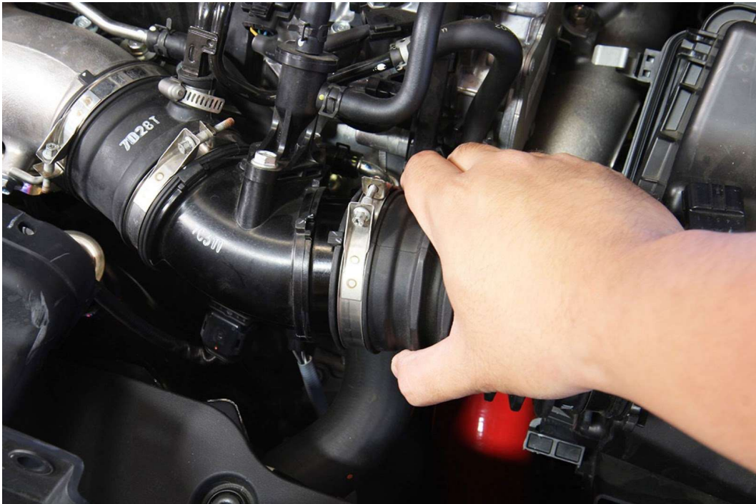
8. Disconnect the intake hose from the purge jet housing.
