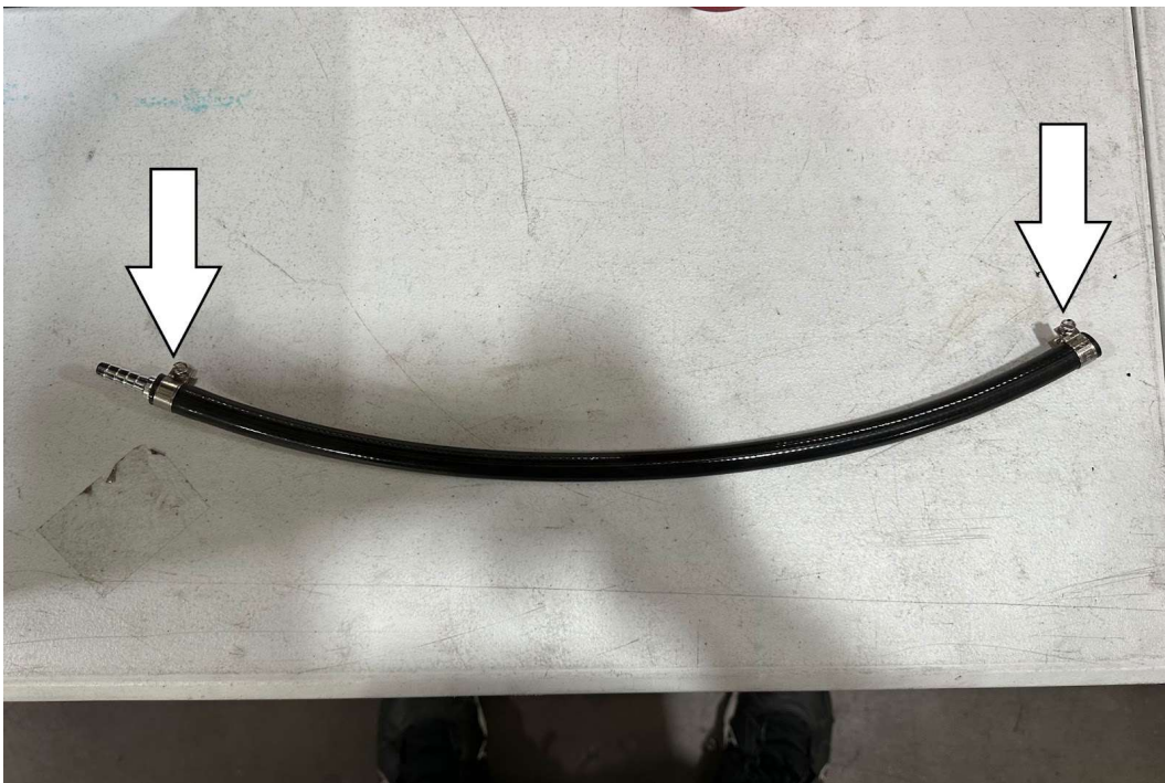
16. Assemble the 13" long heater hose with the two provided FIC-12 clamps and the 5/16" barb fitting as shown in the picture above.
