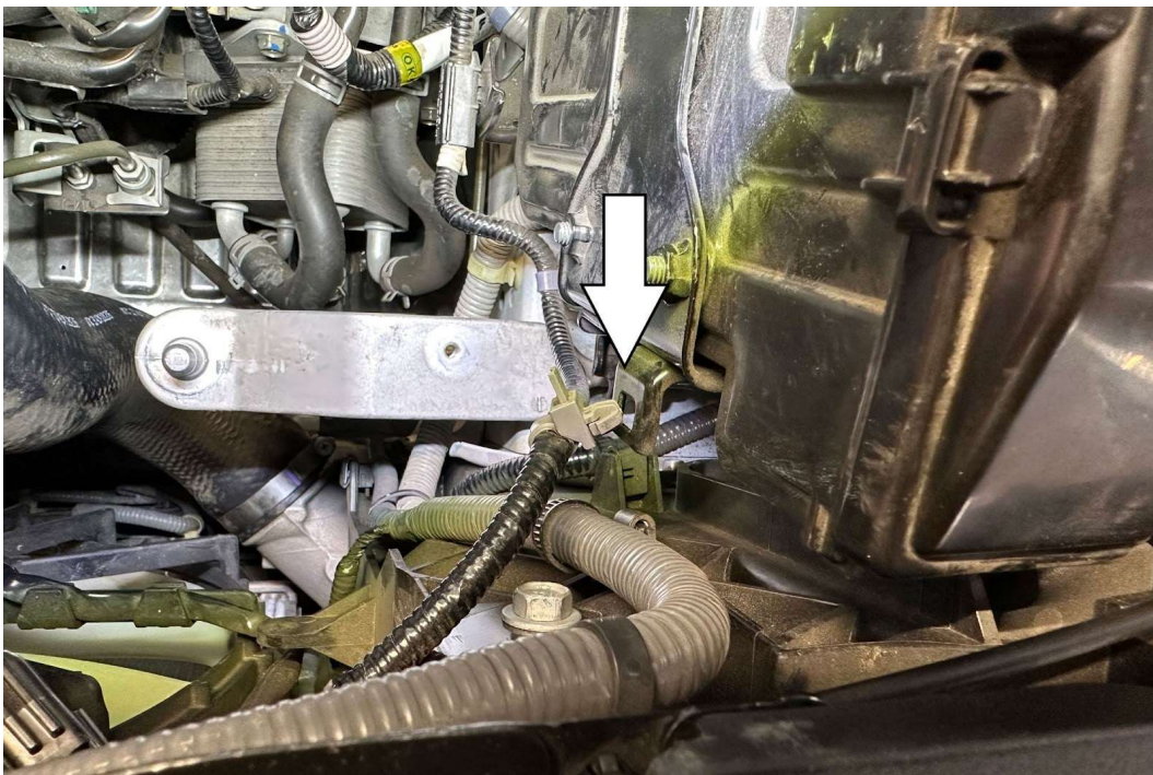
20. Disconnect the plastic clip securing the mass air flow sensor harness to allow the harness to reach the new MAF sensor location.
