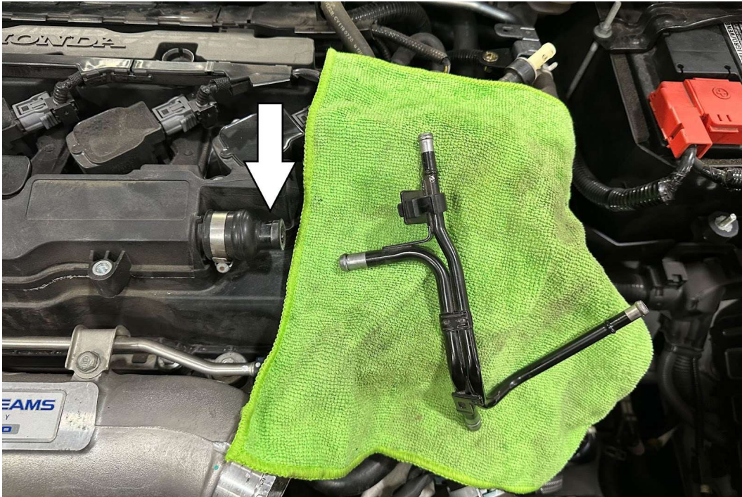
15. Remove the single use clamp from the rubber reducing coupler.
