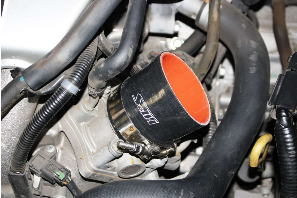
9. Install the straight silicone coupler and T-bolt clamp onto the throttle body.
