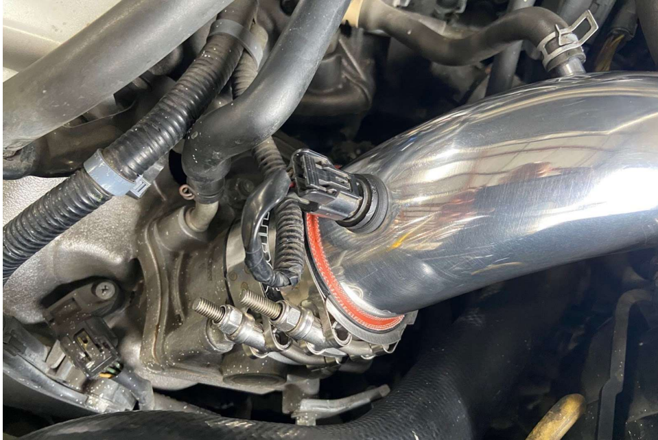
17. Insert the factory air temperature sensor into the grommet.
