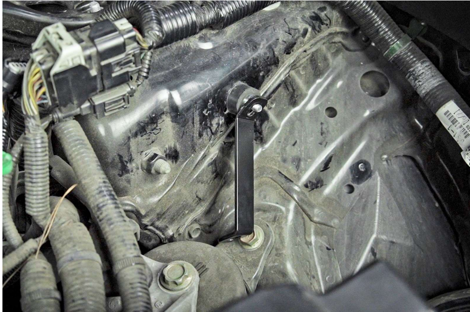
14. Insert the side of the intake bracket with less angle onto the upper vibration mount.
