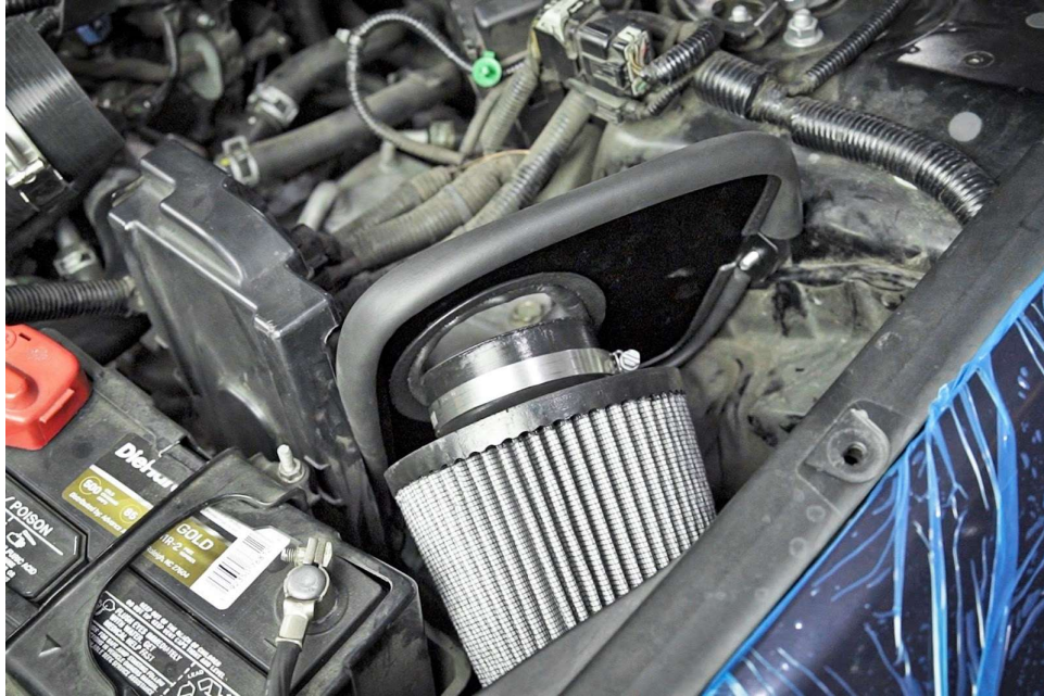
17. Insert the HPS air filter into the engine bay.
