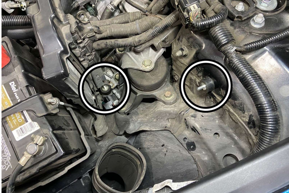
11. Install the provided rubber vibration mounts (2) onto the lower factory air box mount and the upper air box bracket mounting point.
