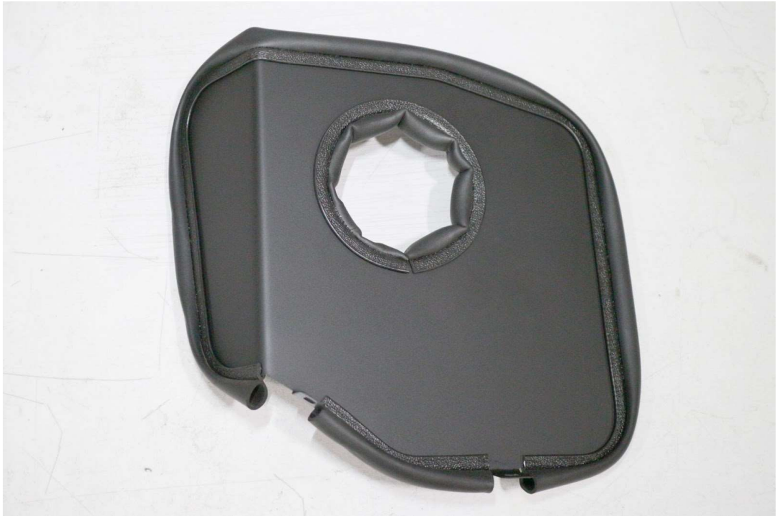
27. Install the bubble edge trim onto the heat shield as shown in the image.
