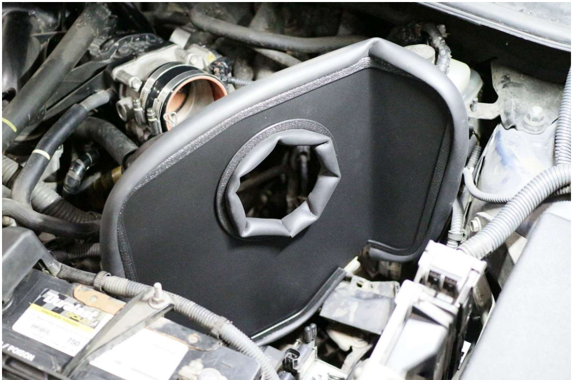
28. Place the heat shield into the engine bay as shown in the image.
