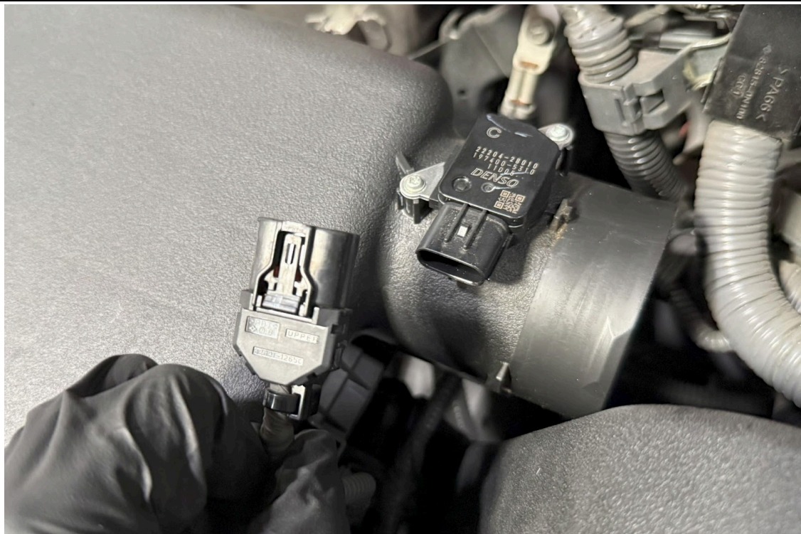
9. Disconnect the MAF sensor.
