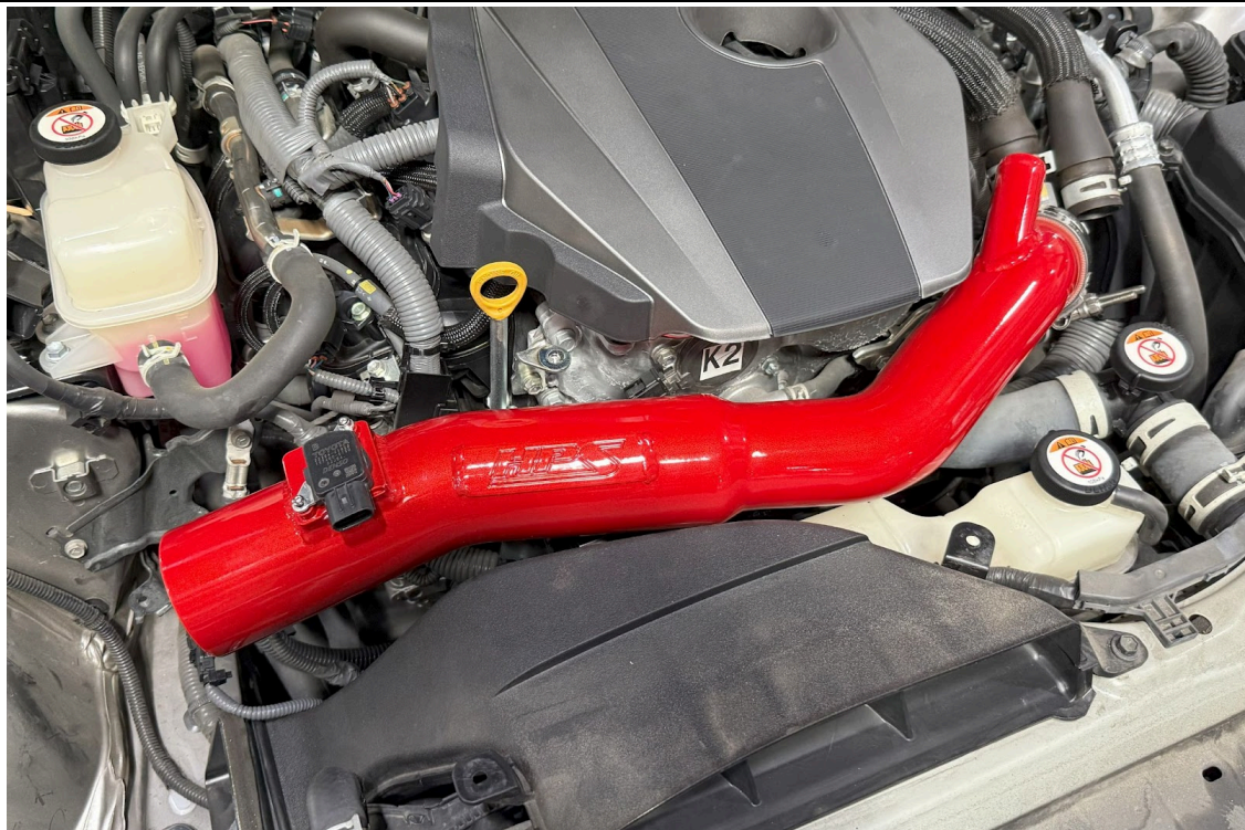
15. Insert the HPS intake pipe onto the silicone reducer.
