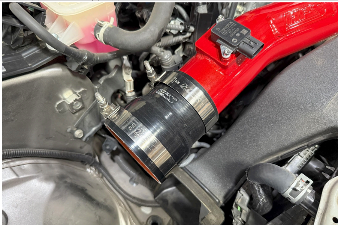
16. Insert the 4" long silicone reducer onto the opposite end of the HPS intake pipe with the remaining T-bolt clamps. Do not fasten the clamps at this time.
