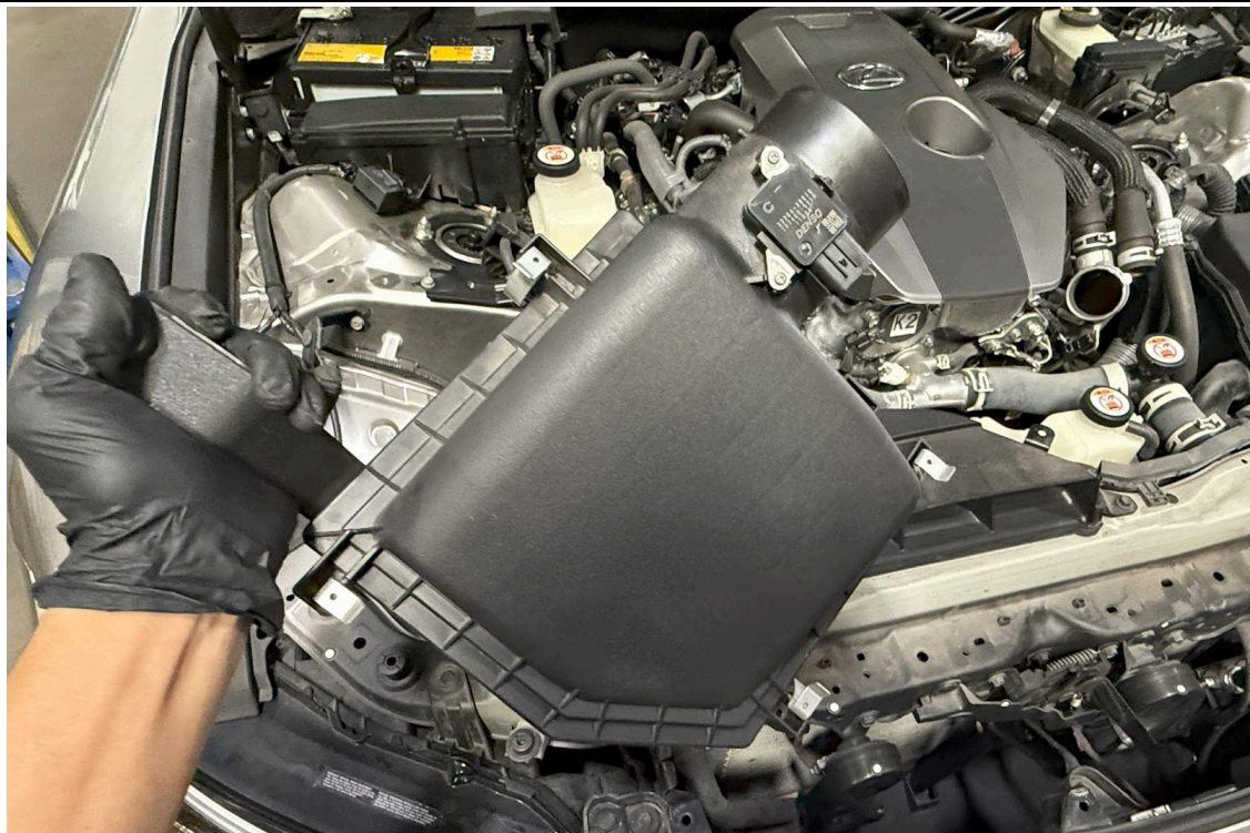
11. Remove the stock air box from the vehicle.
