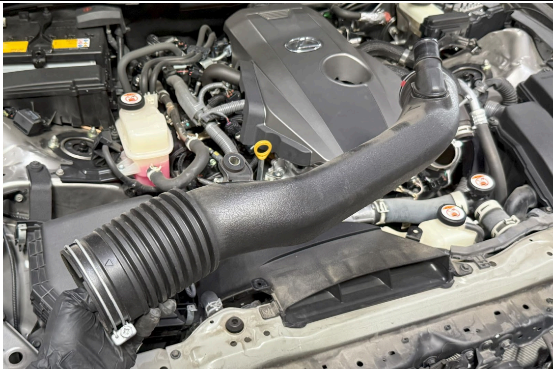
7. Remove the stock intake tube from the vehicle.
