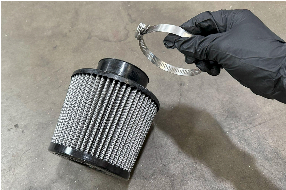
21. Remove the included HPS air filter from its packaging. Then remove the hose clamp from the air filter.
