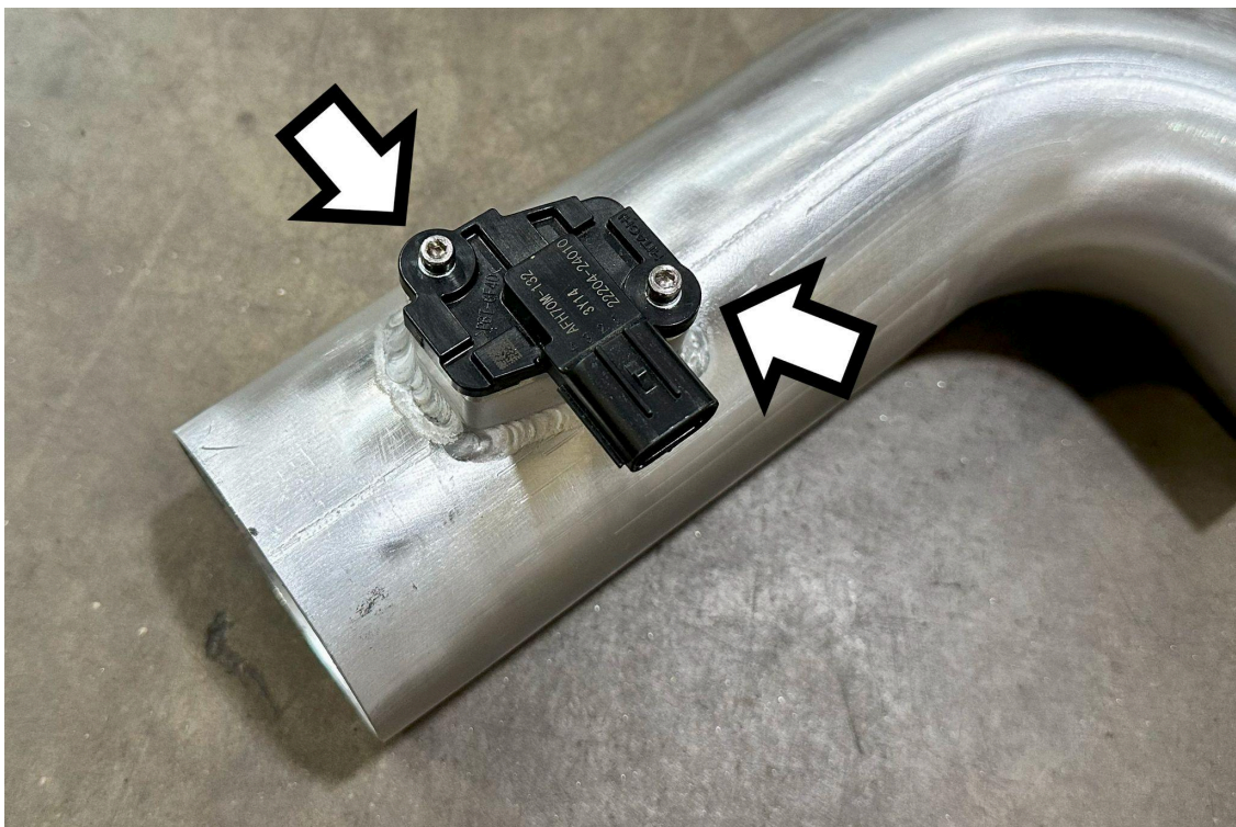
18. Transfer the MAF sensor onto the HPS intake pipe and secure it using the provided M4 screws.
