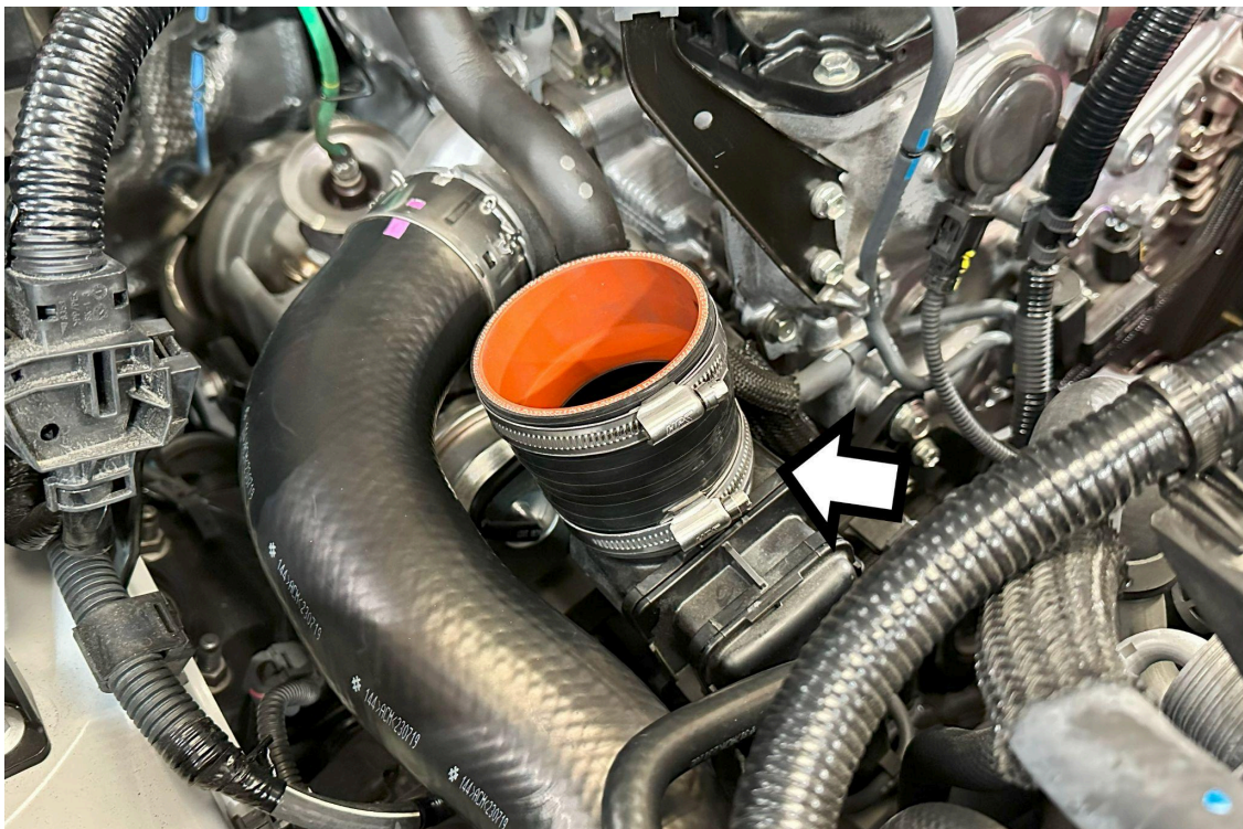
16. Place the provided silicone reducer coupler onto the turbo inlet and secure it using one of the included embossed hose clamps. Place the second embossed hose clamp onto the opposite end of the silicone reducer coupler in preparation for the intake pipe to be installed.
