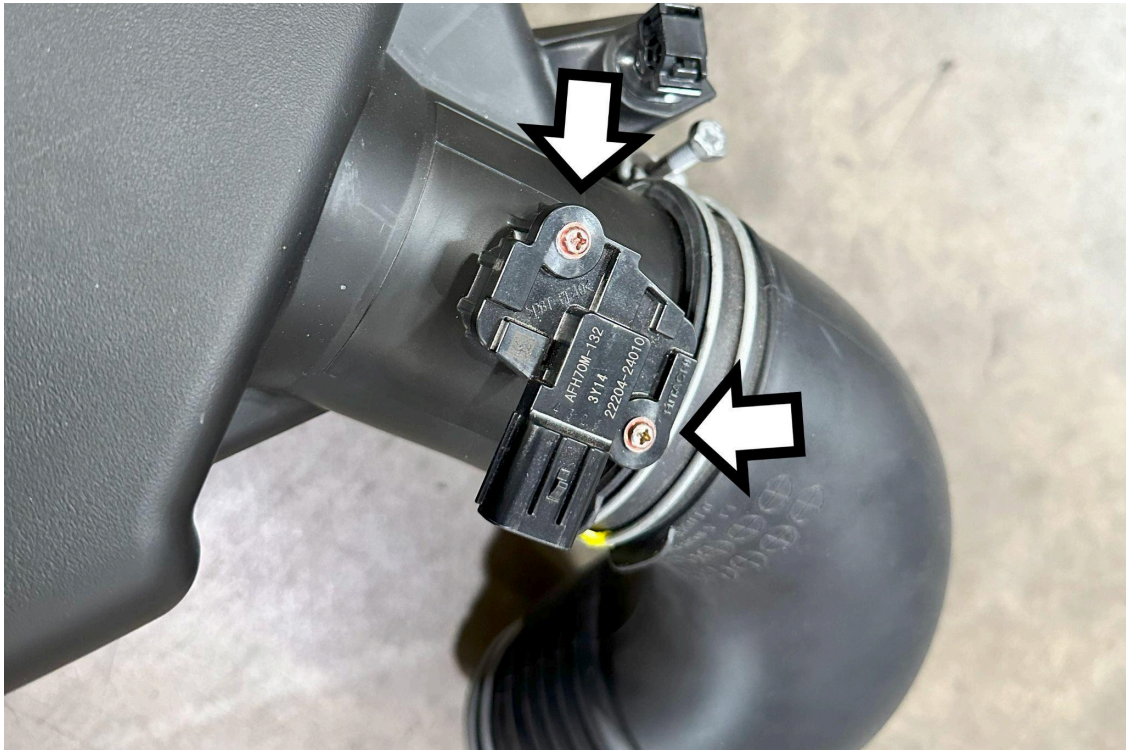
17. Use a Phillips screwdriver to remove the MAF sensor from the stock air box.
