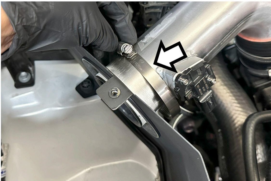
22. Slip the hose clamp over the intake pipe as shown.
