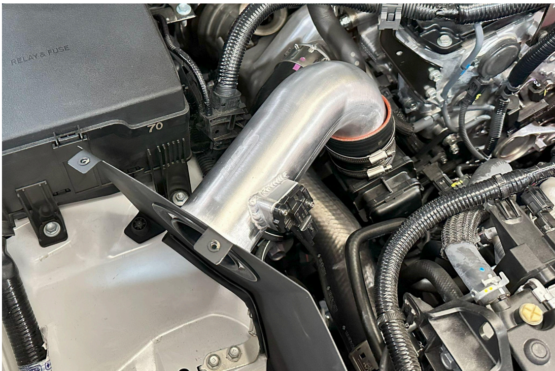
20. Insert the short side of the HPS intake pipe into the silicone reducer coupler. Clock the pipe so that the MAF side of the intake pipe is in line with the opening on the main heat shield.
