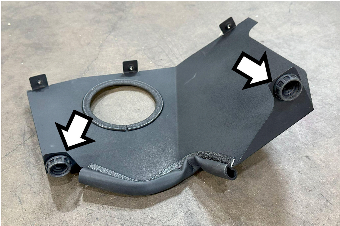
9. Install the rubber grommets onto the mounting points of the main heat shield.
