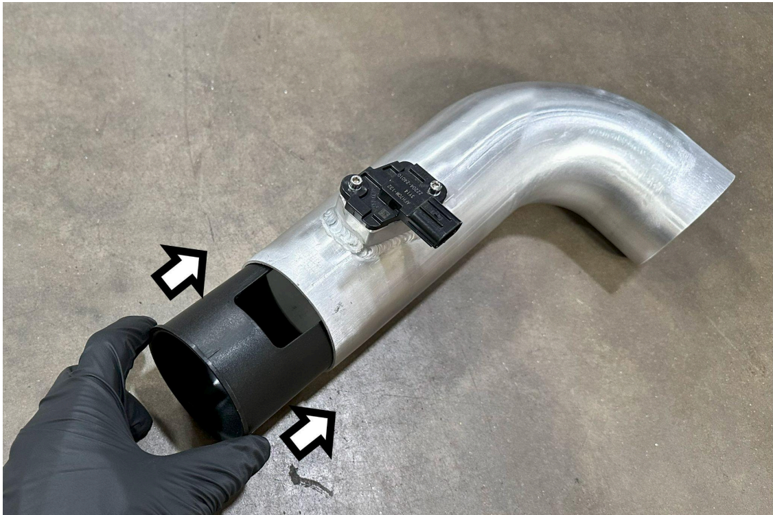
19. Insert the plastic sleeve into the intake pipe in the orientation shown.
