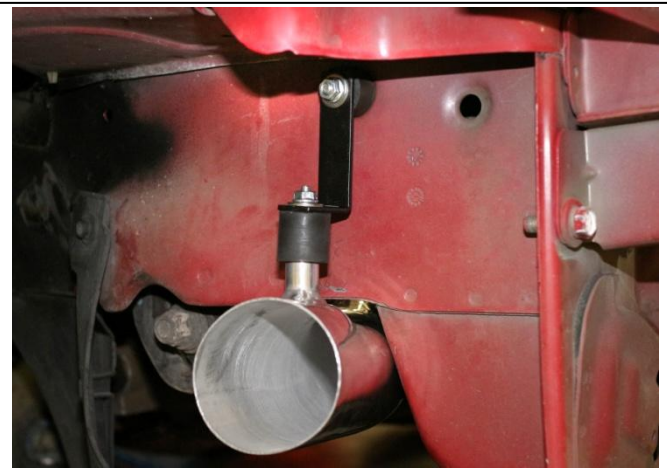
19. Install the cold air bracket (shorter bracket) with the included nuts and washers.
