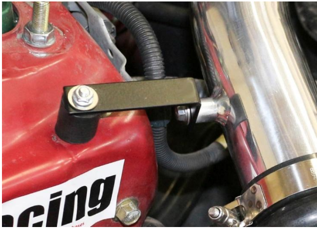
12. Install the intake bracket (longer bracket) with the provided nuts, bolts, and washers.
