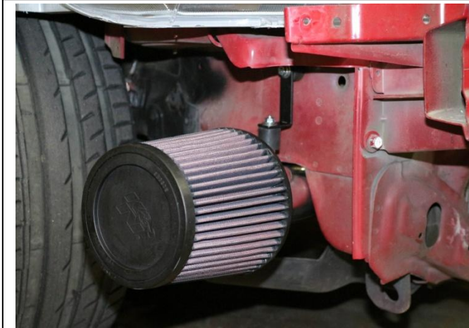
20. Install the air filter onto the cold air pipe.
