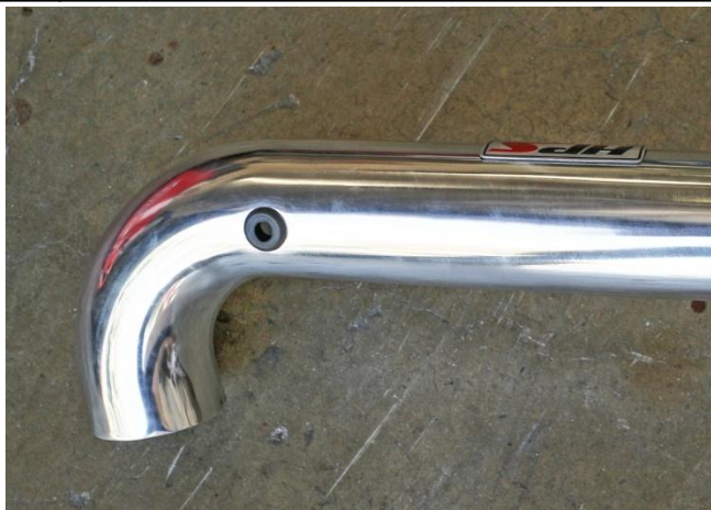
10. Install the rubber grommet onto the port at the back of the intake.
