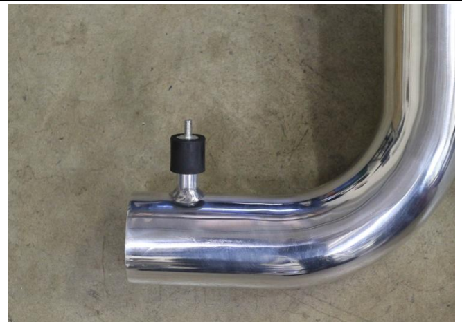
17. Install the 1" rubber mount onto the cold air intake pipe.
