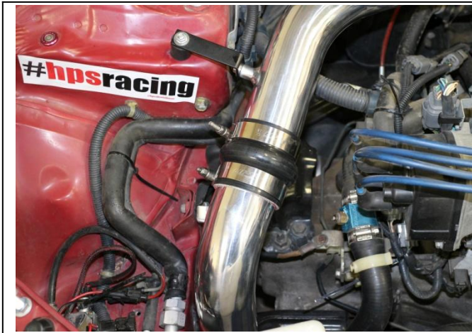
18. Install the cold air intake pipe onto the hump coupler.
