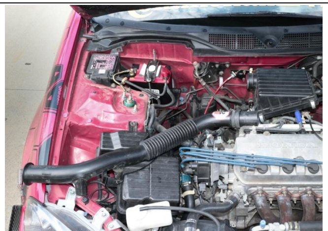
3. Remove the air tube from the engine bay.
