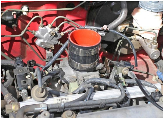
8. Install the silicone reducer onto the throttle body with the included t-bolt clamps.
