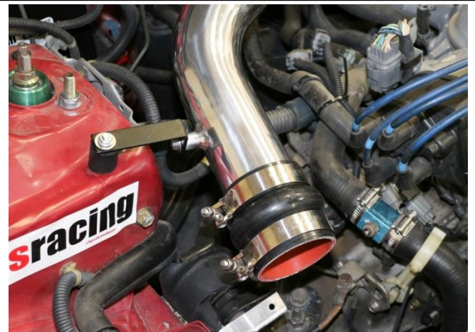
15. Install the hump coupler and t-bolt clamps onto the intake pipe.
