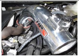
17. Plug in the MAF sensor. Reinstall the breather hose onto the intake pipe. At this point, you can secure the 3" hump coupler to the end of the pipe with one of the T-bolt clamps included.
