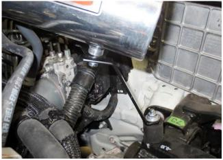
16. Install the mount onto the factory air box mounting plate. Use the included "S" bracket to brace the intake, using the supplied washer and 16mm long 6mm hex bolt. Sandwich the emission sensor bracket between the intake and "S" bracket and tighten down using the supplied washer and 6mm nut.
