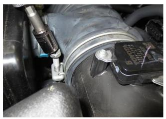
7. Using a 10mm socket or Phillips (cross) screwdriver, unscrew the clamp from the intake hose.
