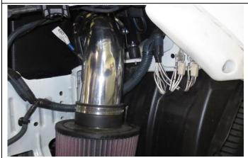
20. Install the rubber vibration mount and bracket, securing the bracket to the mount with the supplied 6mm nut and washer. Slide the pipe into the opening and loosely fit the 12mm long, 6mm bolt and washer through the bracket to the pipe. Install the HPS filter to the end of the pipe.
