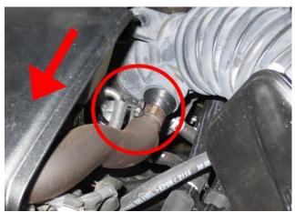
10. Loosen the spring on the breather hose connected to the air hose, then pull the breather hose towards the front of the car to separate it from the main air hose.
