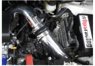
21. Be sure to place the last T-bolt clamp over the hump coupler, and slide the cold air extension pipe into the coupler.
