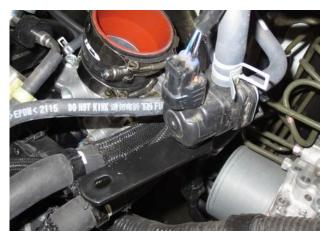
14. Install the supplied bracket using the factory screw.
