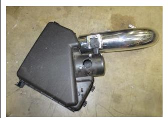
15. Remove the MAF sensor from the factory air box and install it onto the HPS pipe with the included M4 Allen Head bolts. At this point, you can place the intake onto the throttle body without tightening it.
