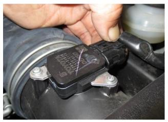
6. Disconnect the mass air flow (MAF) sensor plug.
