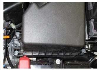
8. Unbuckle the three clips to to remove the top half of the air box.
