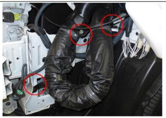
19. Remove the 2 bolts on the top and the plastic clip circled in the image. Once the bolts are removed, you can remove the tube from underneath.
