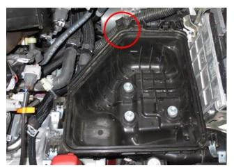
9. Remove the clip holding the harness circled above. Then use a 10mm socket to remove the three bolts holding in the remainder of the factory air box.
