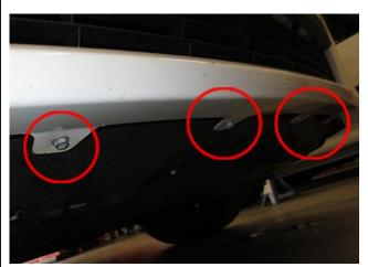
4. Remove the bolts underneath the bumper with a 10mm socket. There are a total of 8 identical bolts along the edge of the bumper.
