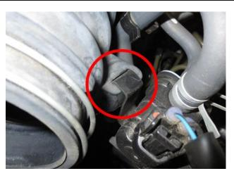
11. Remove the sensor bracket from the air hose by pulling up. Once the bracket is removed, you can remove the air hose from the throttle body by removing the spring clip.
