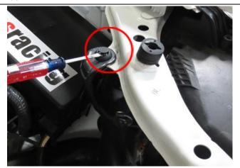
18. Remove the clip holding the air snorkel behind the driver side headlight.
