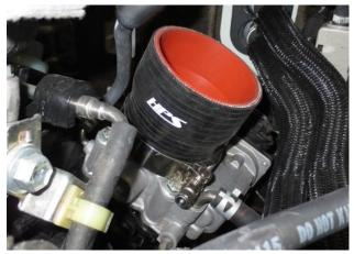
12. Place the reducing coupler onto the throttle body and secure it with a T-bolt clamp.
