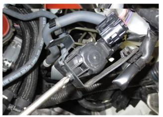
13. Remove the bracket on the emissions sensor with a Phillips (cross) screwdriver.
