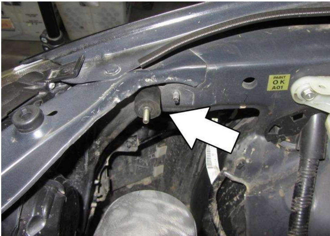
20. Install the 1" rubber vibration mount onto the factory air box mount.
