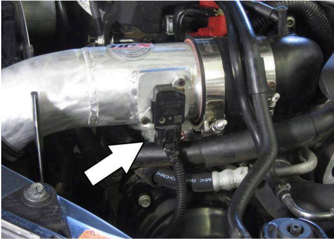
19. Reconnect the MAF sensor.
