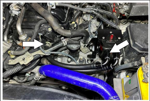
11. Fasten the 90 degree hose end fitting onto the oil catch can. Press the opposite end of the hose onto the port on the intake manifold and secure the hose with the provided embossed hose clamp.
