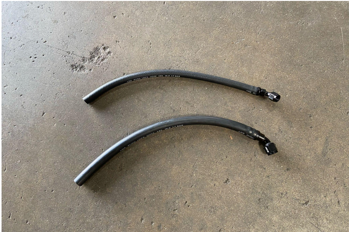
13. Using a small amount of oil to lubricate the hose, push the 45 degree AN hose ends onto the corresponding AN-6 and AN-8 size hoses.
