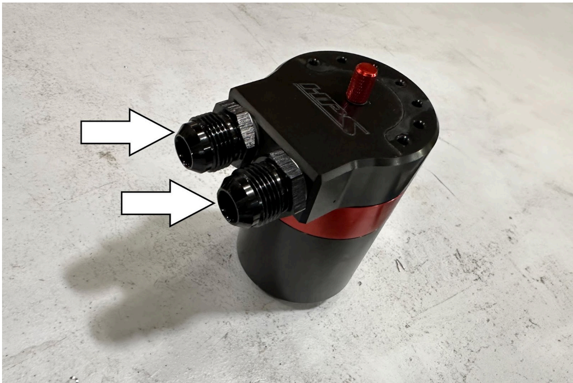
16. Slide the provided crush washers onto the metric side of the provided AN to M16 adapter fittings, then fasten the adapters onto the oil catch can.
