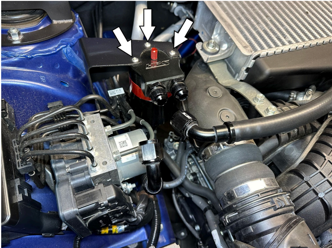
17. Mount the HPS oil catch can to the oil catch can bracket using the three provided M5 bolts.
