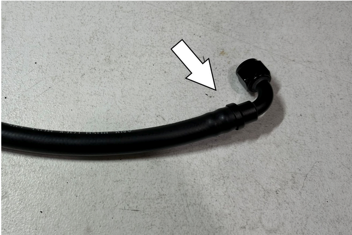
11. Press the 22.5 inch long hose onto the -6, 90 degree hose end fitting.
