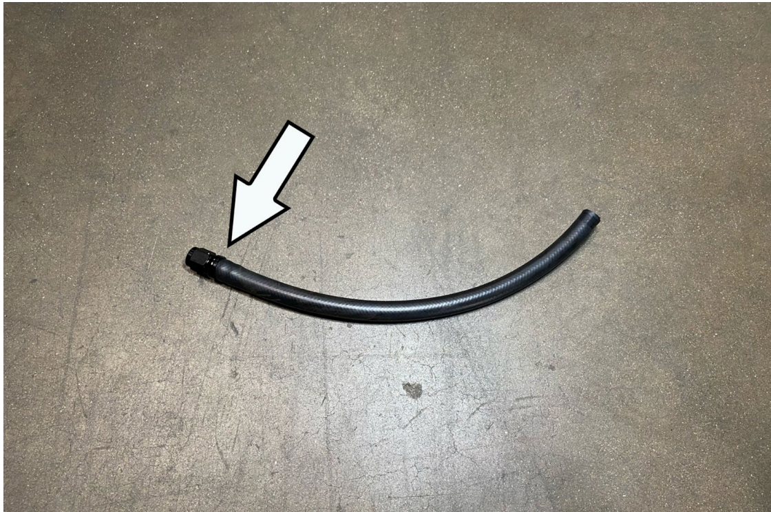
13. Push the longer AN-6 push-on hose onto the AN-6 hose end fitting.
